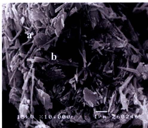
Figure 2.14. SEM images illustrate the morphology of Ranong kaolin minerals, (a) the hexagonal shape of kaolinite, and (b) the tubular shape of halloysite.
