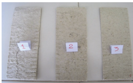
Figure 1 Pieces of rice straw paper (1) 6 mm thickness (2) 4 mm thickness (3) 2 mm thickness
