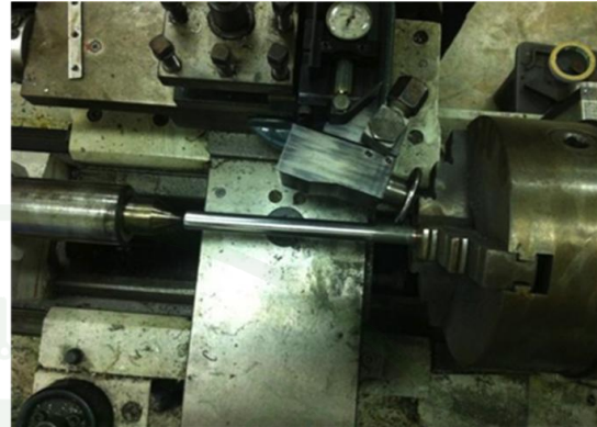
1 = workpiece 2 = deep rolling device
