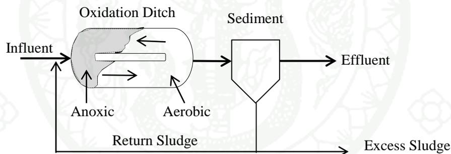
**Figure 11** Oxidation Ditch
