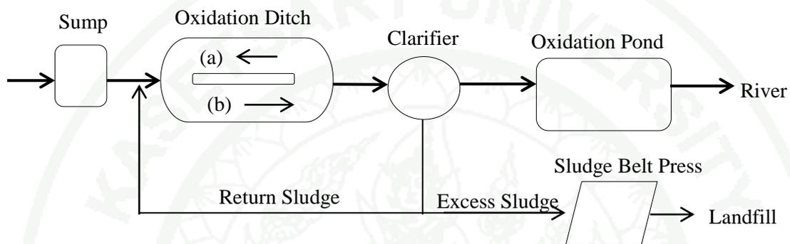
**Figure 14** Phuket wastewater treatment plant.
