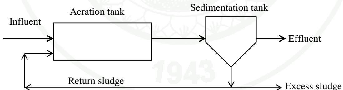
**Figure 3** Extended Aeration Activated Sludge
