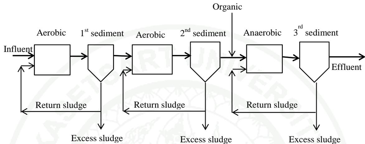
**Figure 8** Remove nitrogen by 3 tanks of sludge
