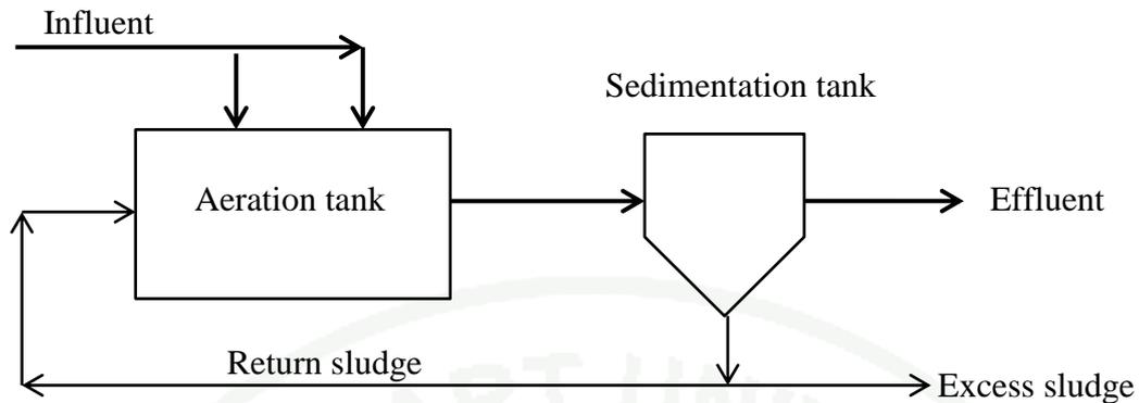
**Figure 2** Complete Mixed Activated Sludge
