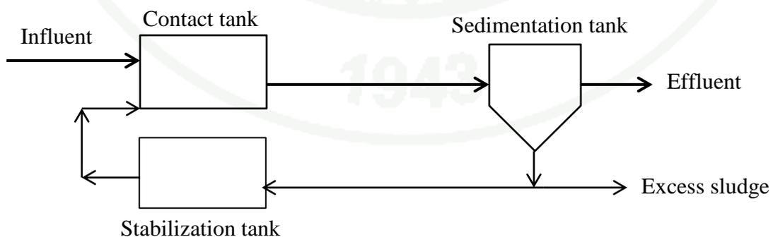
**Figure 5** Contact Stabilization Activated Sludge
