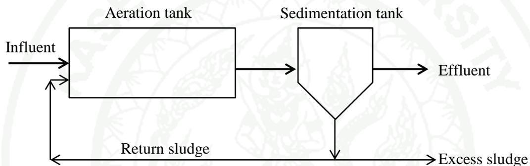
**Figure 1** Conventional Activated Sludge
