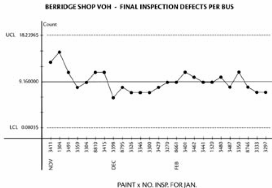
Figure 2.6 The application of Control Chart c at SEPTA's Paint Shop
