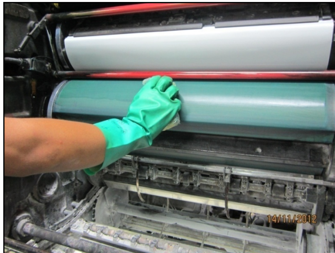
Figure H.1 Cleaning the roller of printing machine
