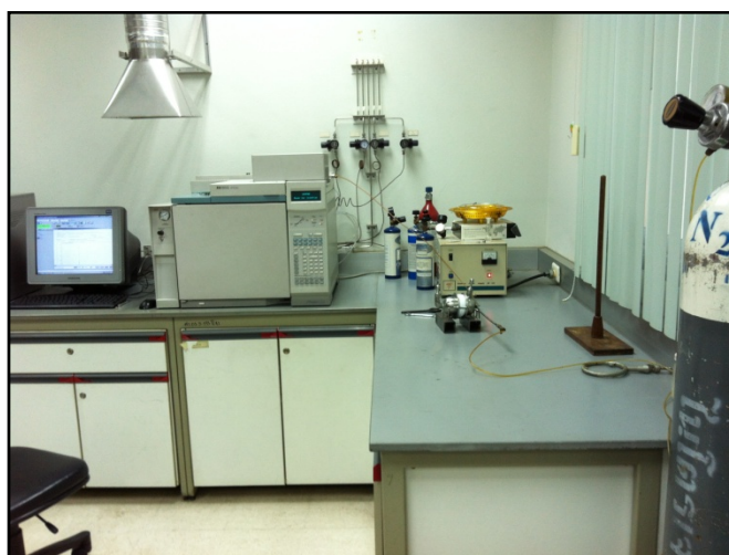
Figure E.2 GC-FID connect to permeation test cell
