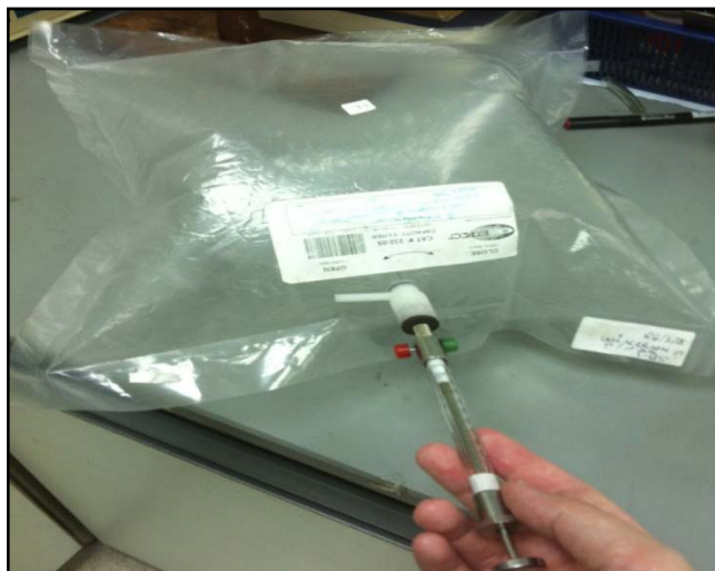
Figure F.1 Injecting known concentration of chemical (n-hexane, benzene and ethylbenzene) into tedlar bag
