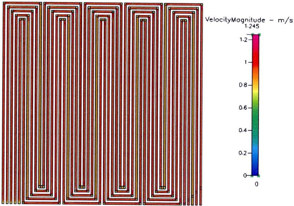
Figure B.43 Velocity distribution at 200 cm 3 /min of 5 channels
