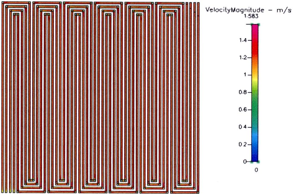
Figure B.37 Velocity distribution at 200 \text{ cm}^3/\text{min} of 4 channels
