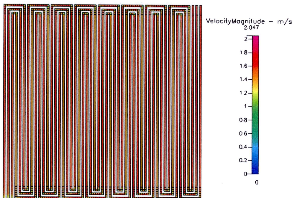
Figure B.31 Velocity distribution at 200 cm 3 /min of 3 channels
