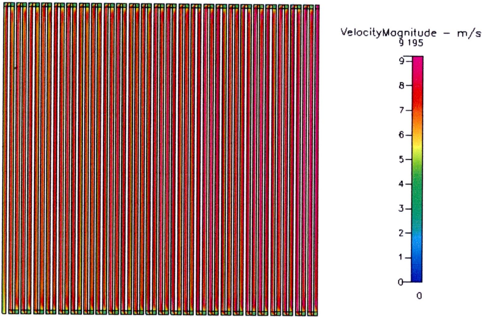
Figure B.75 Velocity distribution at 400 cm 3 /min of 1.2 mm. channel width
