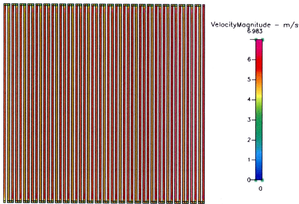
Figure B.55 Velocity distribution at 200 cm 3 /min of 0.8 mm. channel depth
