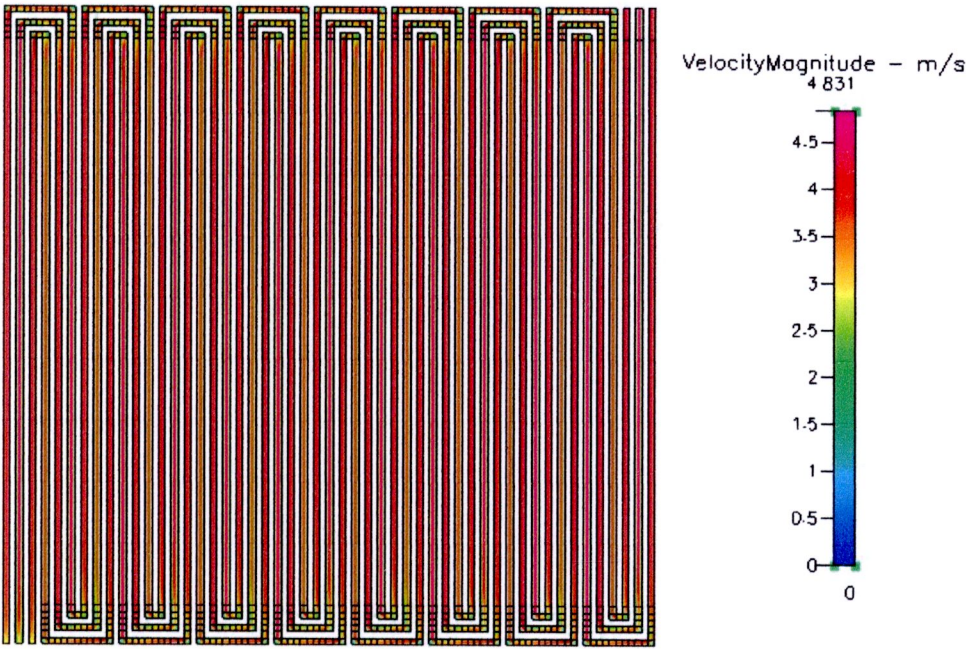
Figure B.35 Velocity distribution at 500 cm 3 /min of 3 channels
