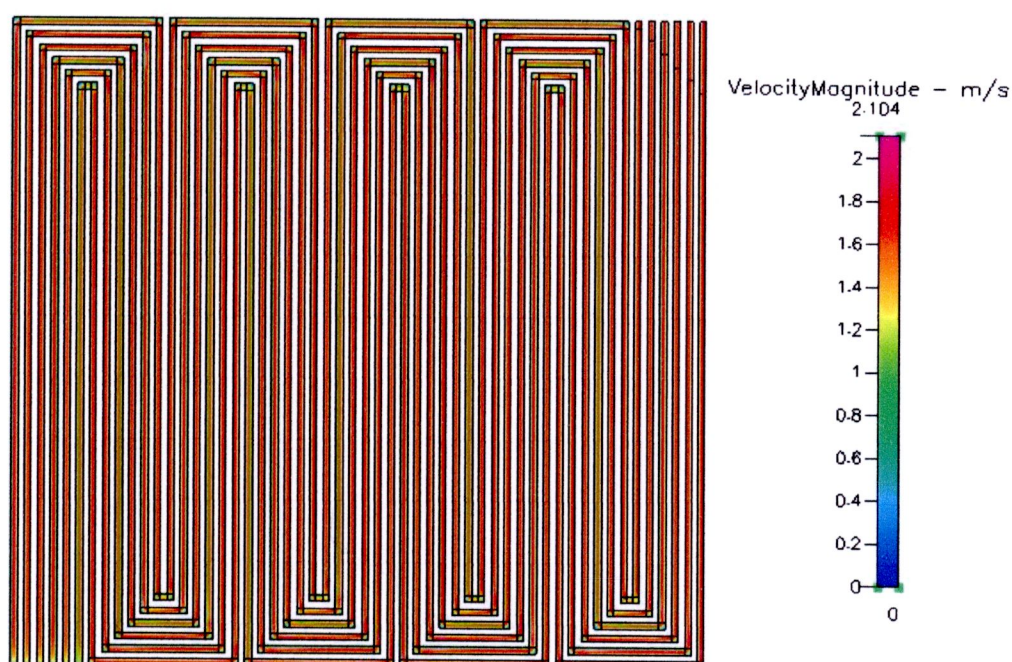
Figure B.51 Velocity distribution at 400 \text{ cm}^3/\text{min} of 6 channels
