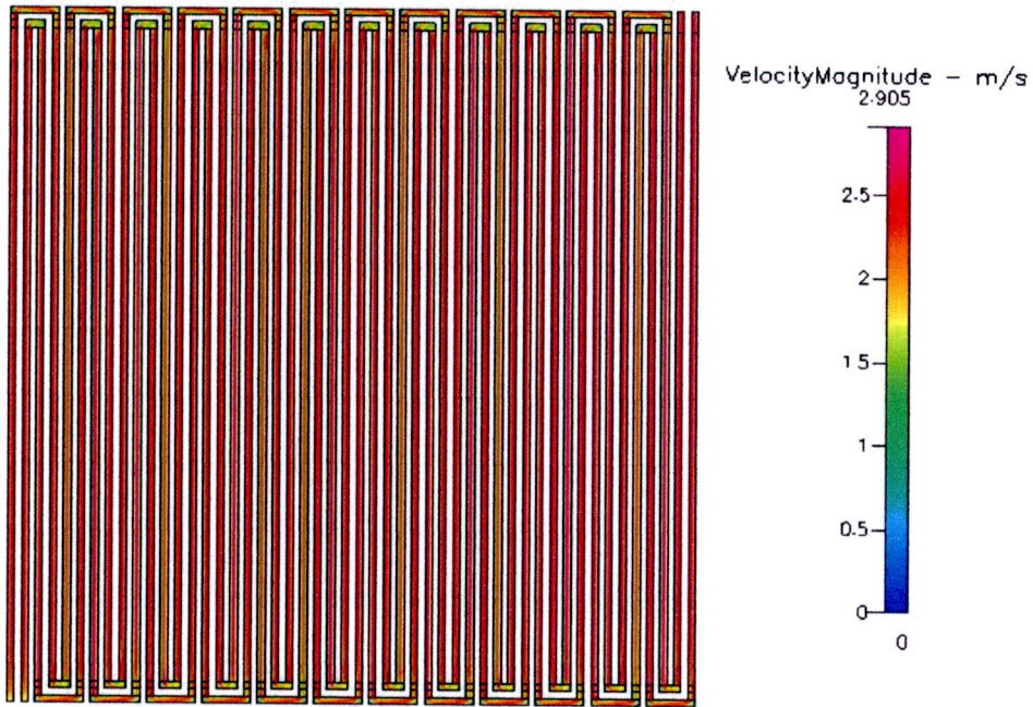
Figure B.25 Velocity distribution at 200 \text{ cm}^3/\text{min} of 2 channels
