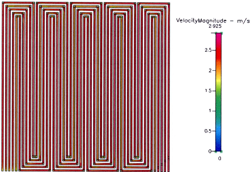
Figure B.47 Velocity distribution at 500 cm 3 /min of 5 channels
