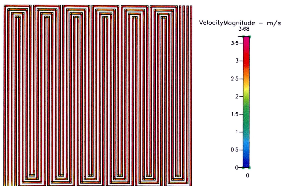
Figure B.41 Velocity distribution at 500 \text{ cm}^3/\text{min} of 4 channels
