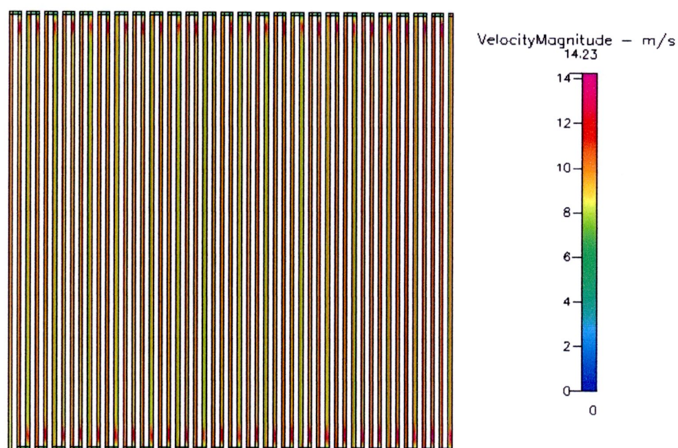
Figure B.69 Velocity distribution at 400 \text{ cm}^3/\text{min} of 0.8 mm. channel width
