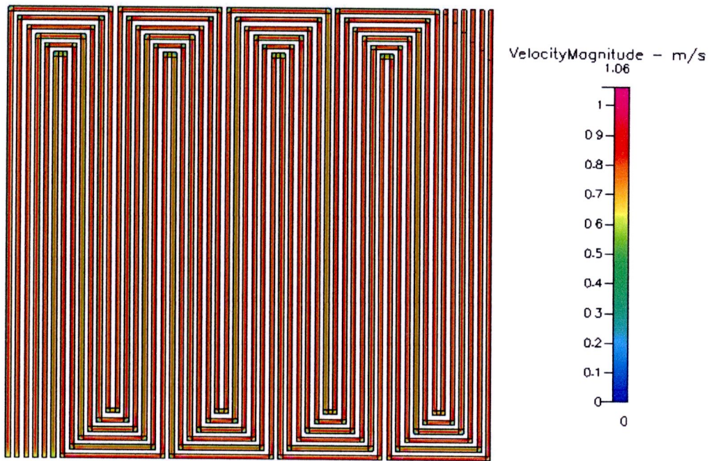
Figure B.49 Velocity distribution at 200 cm 3 /min of 6 channels
