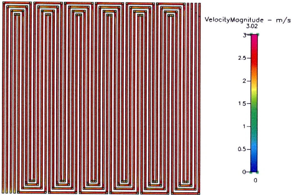
Figure B.39 Velocity distribution at 400 \text{ cm}^3/\text{min} of 4 channels
