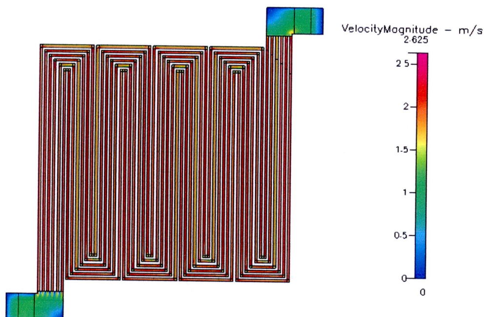
Figure B.113 Velocity distribution at 500 \text{ cm}^3/\text{min} of 90 turn non-fillet manifold
