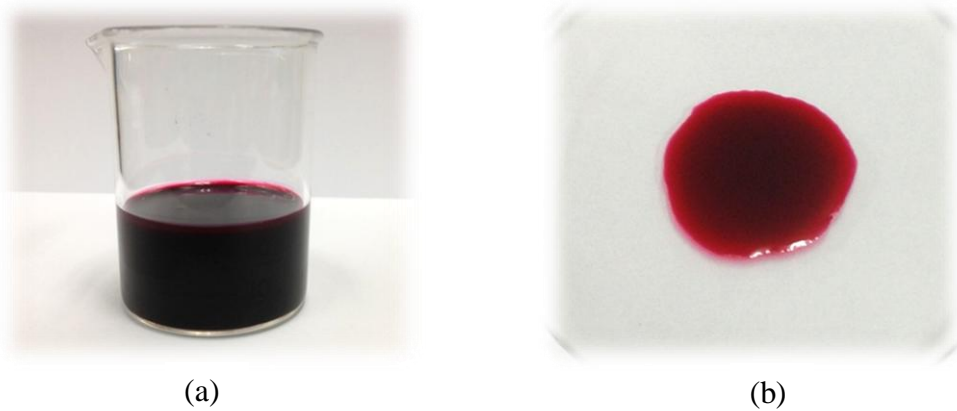
Figure 5.1 Dragon fruit peel colorant extracted from dragon fruit peel; (a) colorant in bulk solution and (b) one drop of colorant
