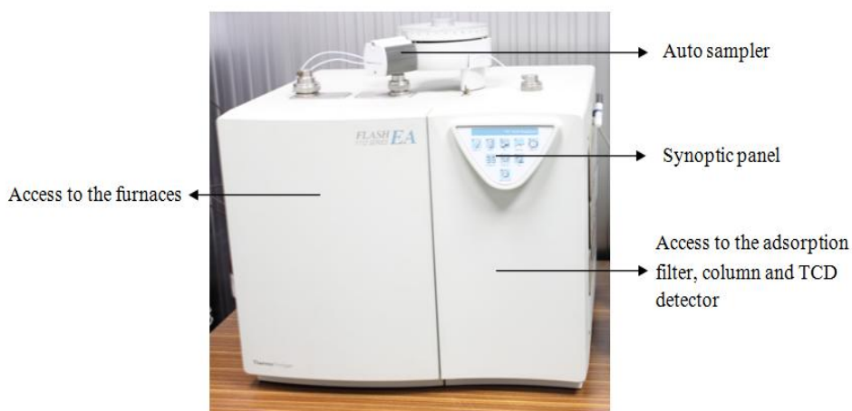
Figure 3.9 A CHONS analyzer used in this study (Thermo Finnigan, Flash EA1112)
