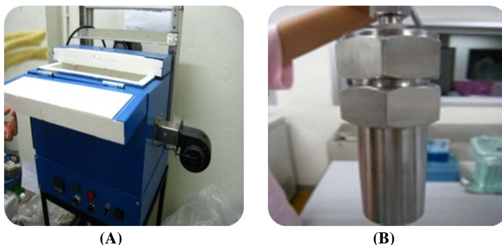
Figure 3.4 The experimental set up apparatus: (A) Furnace and (B) Reactor
