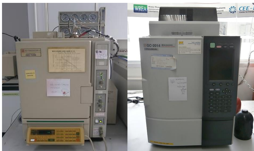
Figure 3.9 Gas Chromatograph (GC-14B and GC-2014, SHIMADZU)
