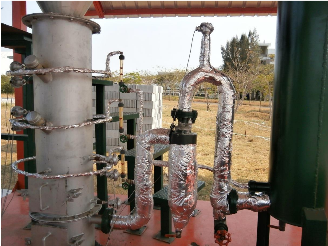
Figure 4.14 The Insulated Piping System and Cyclone
