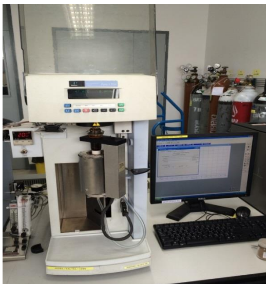
Figure 3.3 Thermo-Gravimetric Analyzer (PerkinElmer, TGA Phyris 1)
