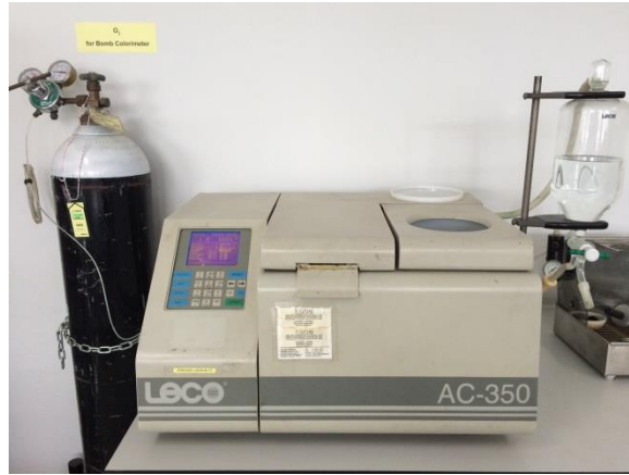
Figure 3.5 The Bomb Calorimeter (LECO AC-350)
