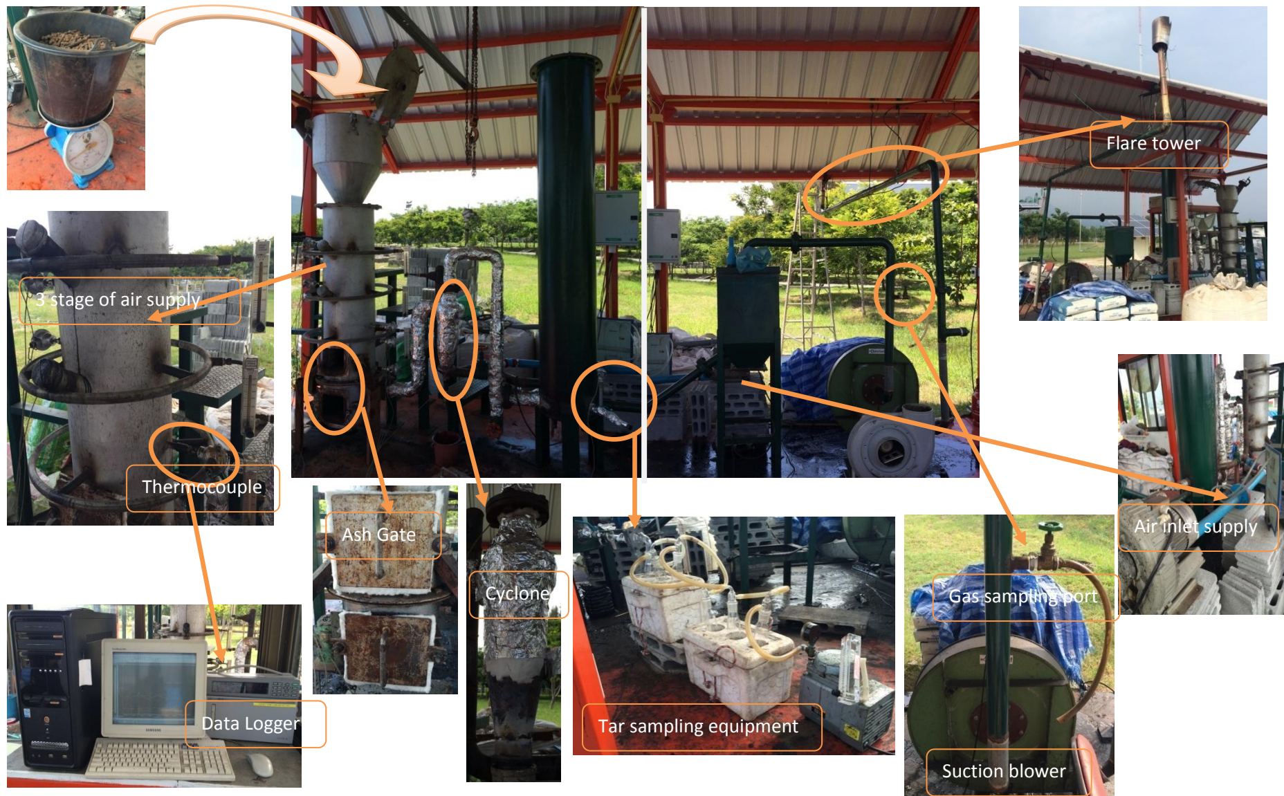
Figure 3.10 Multi-air-stage downdraft gasification system
