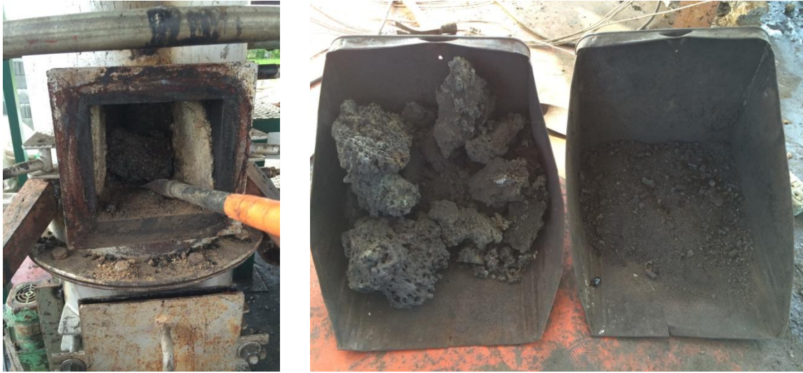
Figure 4.17 The slag in gasifier
