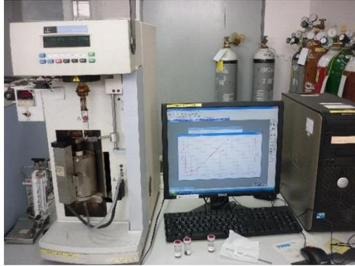
**Figure 3.3** TGA analyzer.
