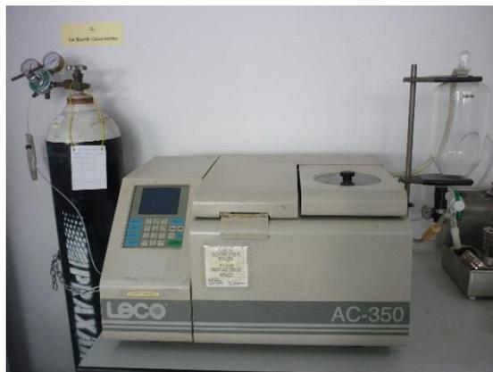
**Figure 3.4** Bomb calorimeter.
