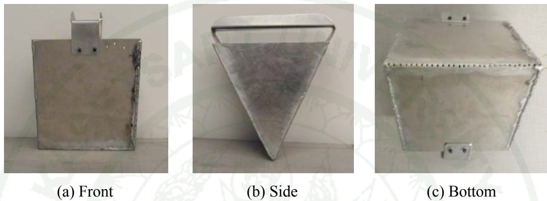
Figure 34 Pluviator from the front, side and bottom views
