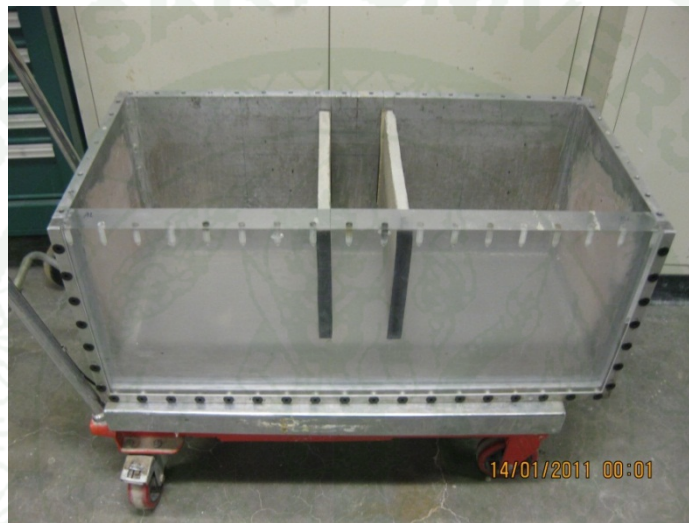
Figure 43 Installation of the soil cement wall into the box
