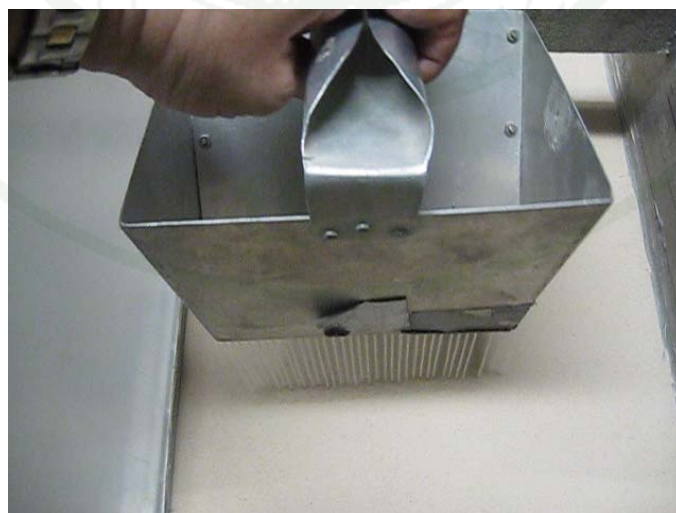
Figure 44 Sand raining using pluviator
