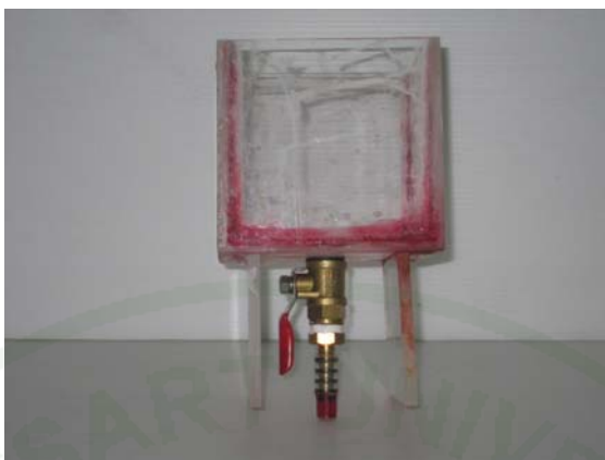
Figure 29 A gasoline storage container
