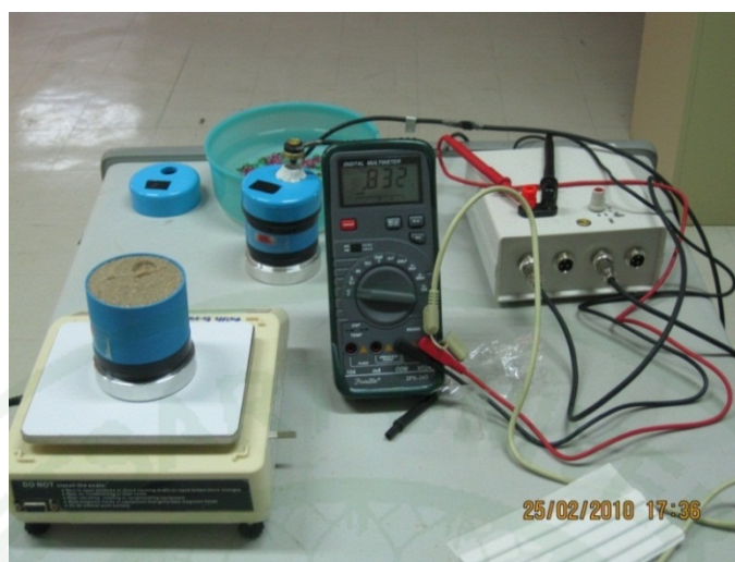
Figure 42 Experimental set up for suction-monitoring
