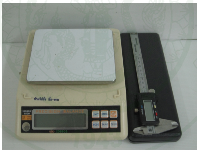
Figure 27 Devices to measure the changes in the dimensions and water content of the samples
