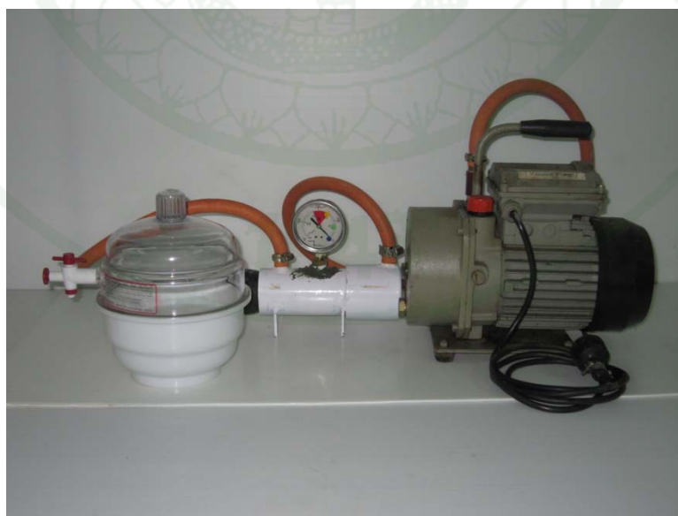
Figure 23 The vacuum chamber and vacuum pump used to saturate the tensiometer
