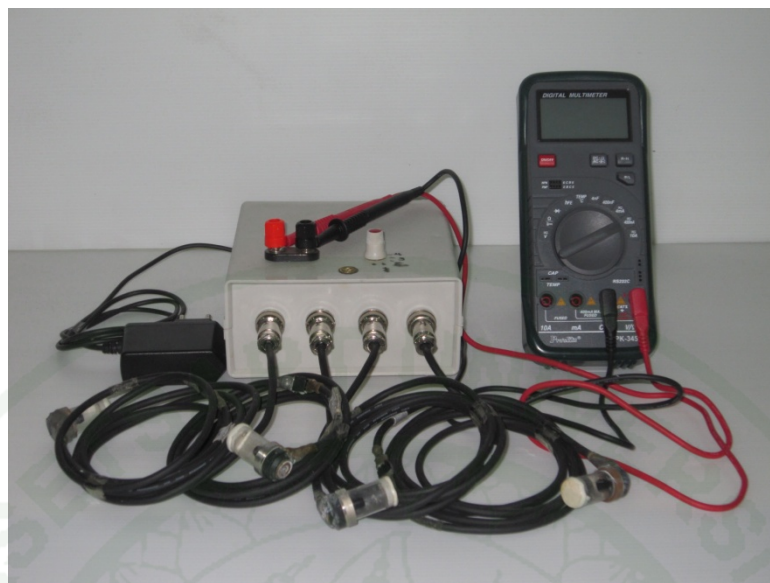
Figure 24 Experimental set up for suction monitoring
