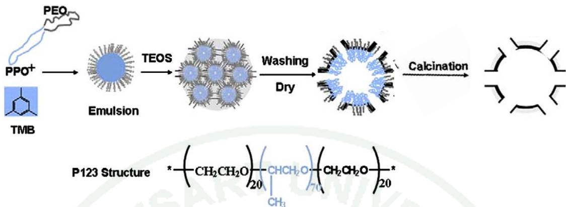
Figure 5 Schematic of the pore size modification by using TMB
