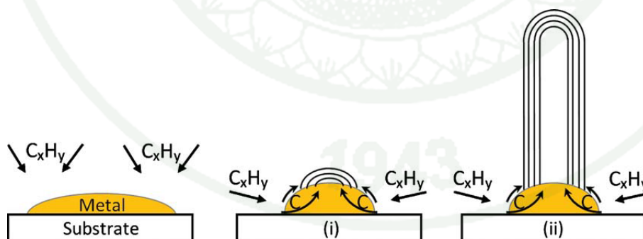
Figure 8 Schematic of base-growth mechanism
