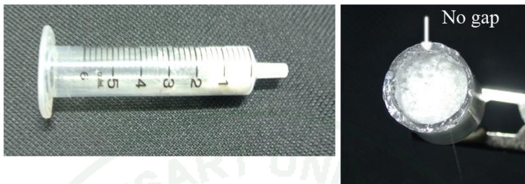
Figure 11 C-18 silica monolith left three months after fabrication. No shrinkage and no gap between the wall and the monolith inside.
