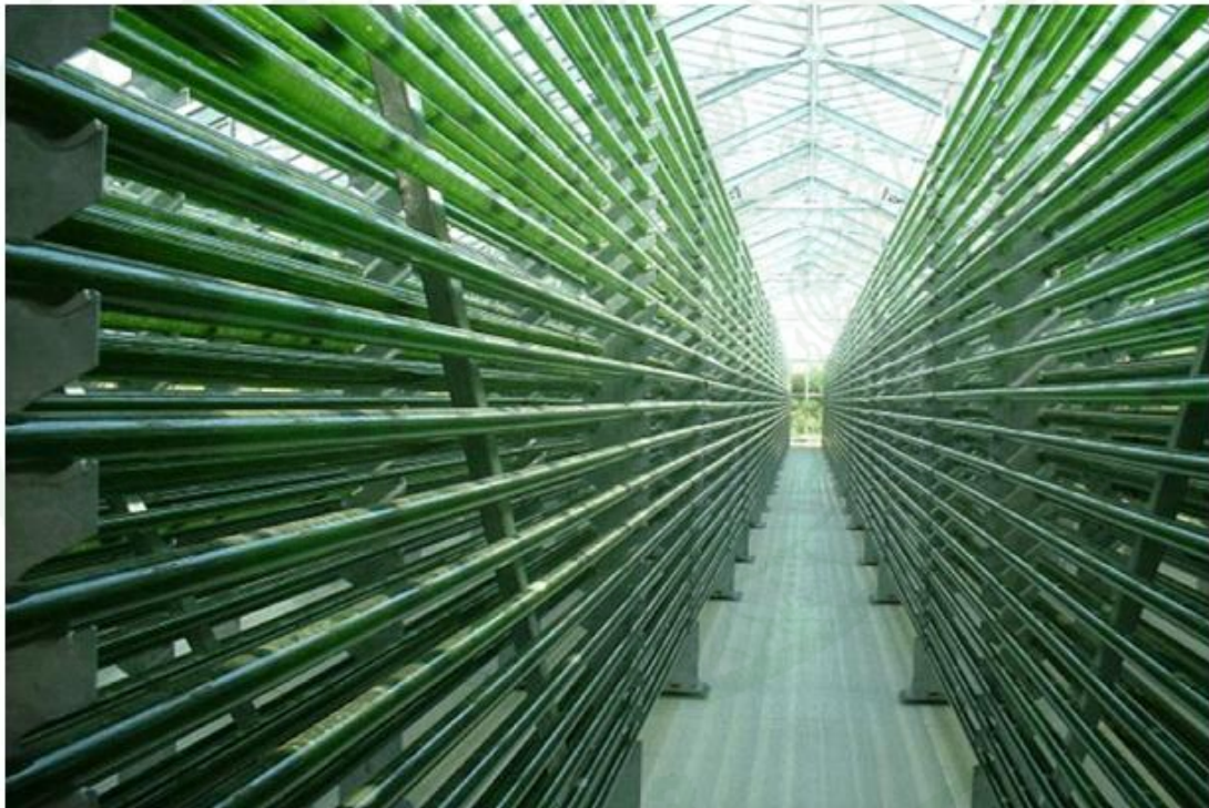
Figure 2 Schematic photobioreactor design, as follows a horizontal tubes.
