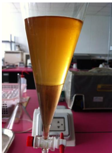
Figure 3.3 Phase separation of biodiesel and another phase in separating funnel after esterification
