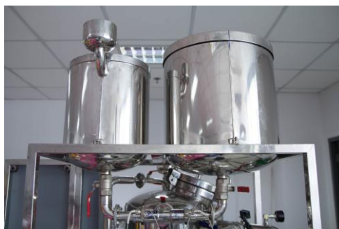
Figure 4.2 Raw material tanks (methanol and coconut fatty acid tanks)
