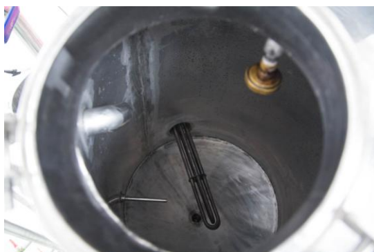
Figure 4.4 Electric heater and thermocouple in the mixing tank
