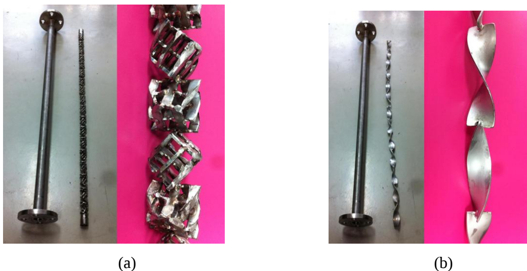
Figure 4.6 Static mixers and their element pieces (a) SMX mixer and (b) Kenics mixer
