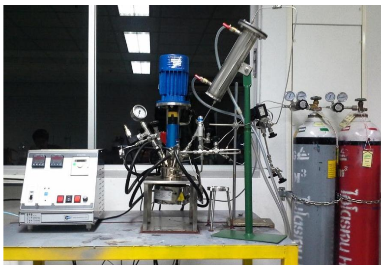
Figure C.1 The high pressure autoclave reactor (semi-continuous proces)
