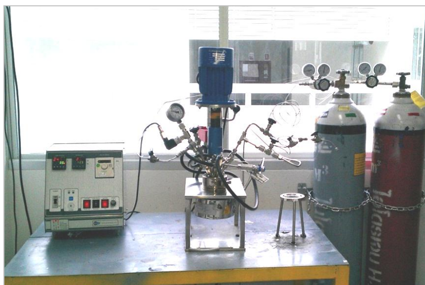
Figure 3.2 Mechanically stirred stainless steel autoclave.
