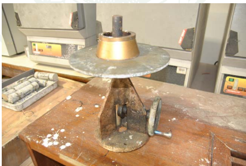
Appendix Figure B4 Flow test set
