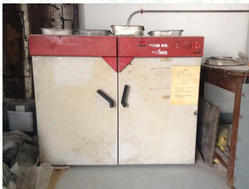
Appendix Figure B12 Hot air oven.
