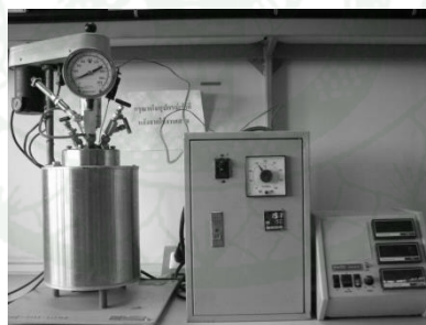
Figure 14 Hydrothermal reactor with controlled temperature and speed, (Model 4516 M PARR).
