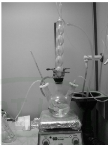
Figure 15 Reactor for kinetics analysis of phenolic compounds.
