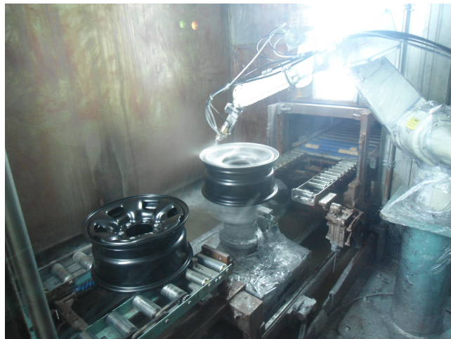
Fig. 10 Top coating (painting) operation
