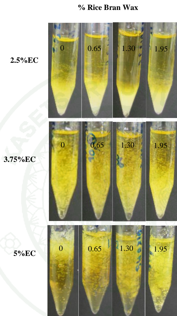
Figure 32 Effect of oleogelators on salt sedimentation in rice bran oil oleogel after storage at 90°C for 12 h.
