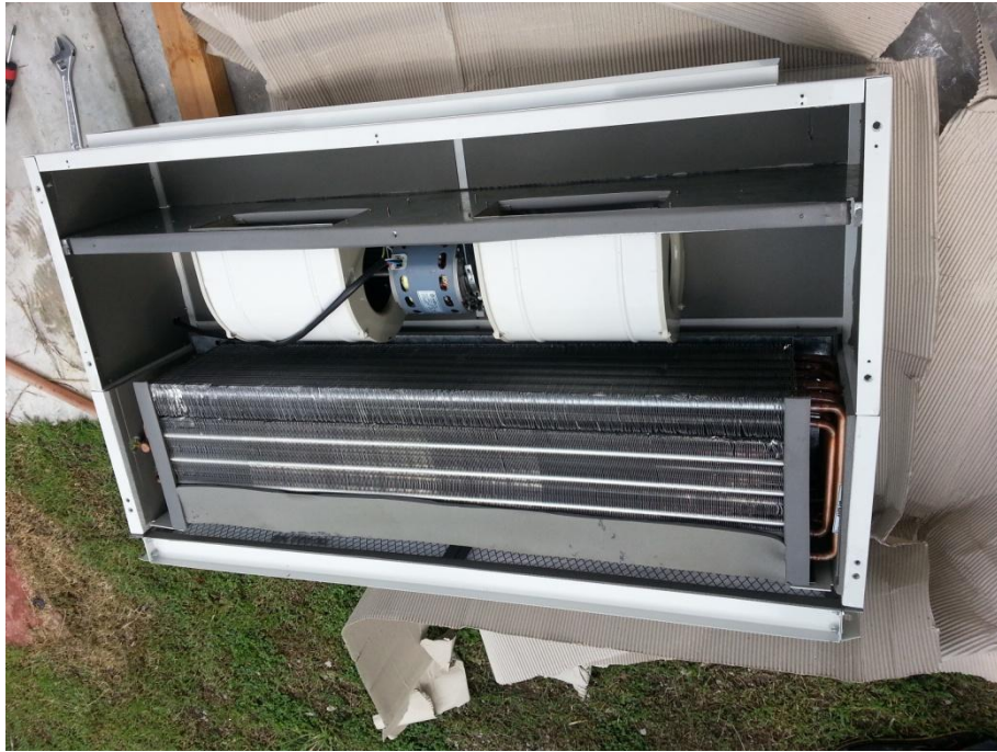
Figure A.2 A photograph of chilled water tubes inside heat pipe run-around-coil heat recovery.
