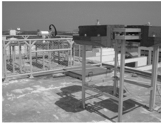
Figure 3.2 A photograph of the daylight and solar radiation station.
