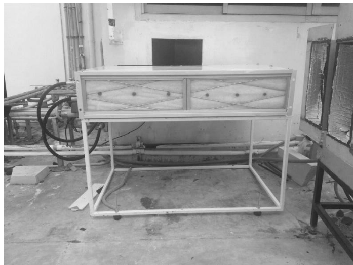
Figure 3.11 A Dehumidification unit (Heat pipe run-around-coil heat recovery).
