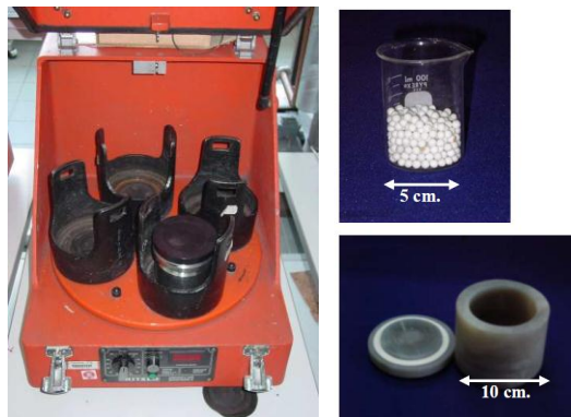
Figure 3.6 Equipment for mashed (planetary mill)
