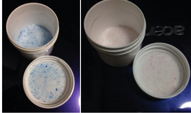
Figure 3.5 Silica-gel (0.1-0.7mm) before and adsorbed humidity after 1 day
