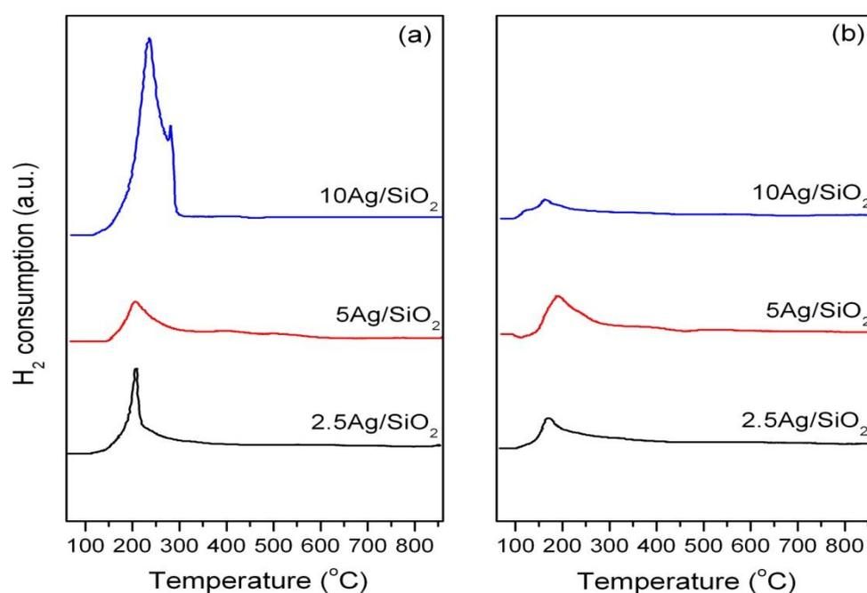
**Figure 4.5** TPR profiles of silver doped on silica support catalyst at different silver loadings: (a) typical impregnation technique and (b) microwave-assisted technique.
