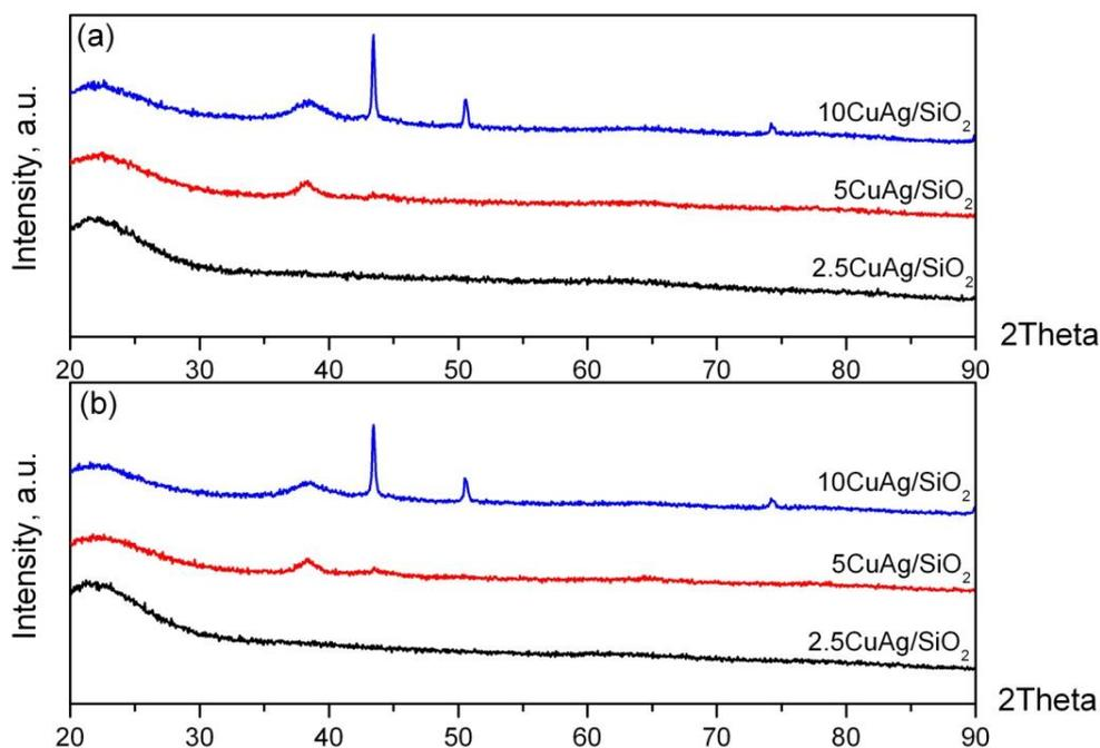
**Figure 4.3** XRD patterns of bimetallic copper and silver doped on silica support catalyst after being reduced in 10% v/v H<sub>2</sub> in N<sub>2</sub> at 300°C for 3 hours at different total metal loadings: (a) typical impregnation technique and (b) microwave-assisted technique.
