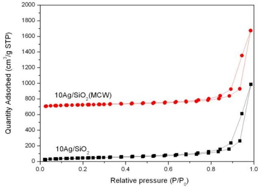
**Figure B.9** Adsorption and desorption isotherms of 10 wt.% silver doped on silica support: (■) typical impregnation technique and (●) microwave-assisted technique.
