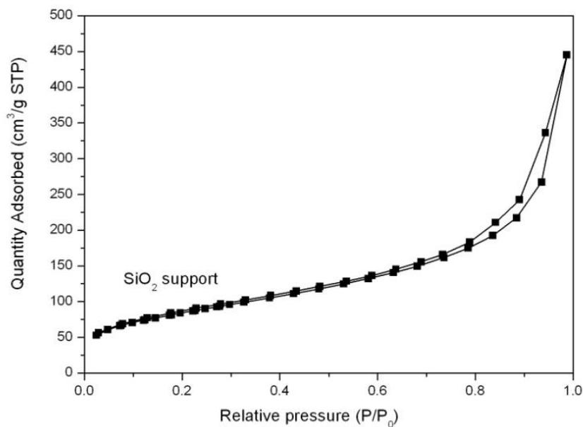
**Figure B.1** Adsorption and desorption isotherms of silica support.
