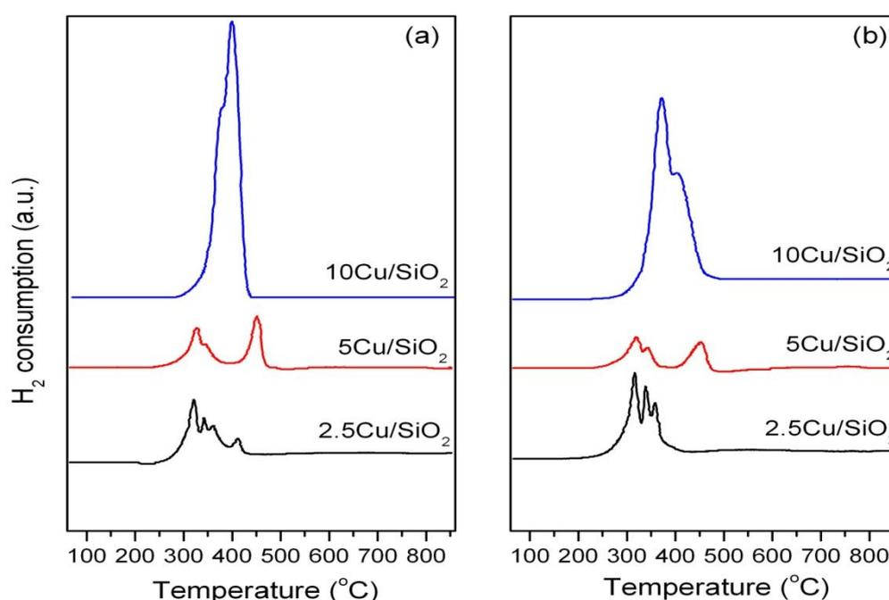
**Figure 4.4** TPR profiles of copper doped on silica support catalyst at different copper loadings: (a) typical impregnation technique and (b) microwave-assisted technique.
