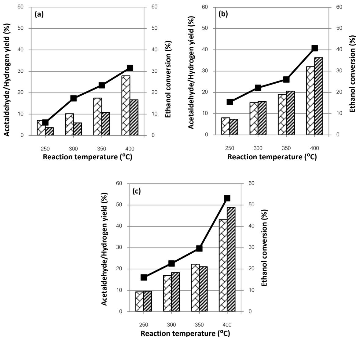
**Figure 4.12** Ethanol conversion, acetaldehyde and hydrogen yield as a function of reaction temperature for ethanol dehydrogenation reaction over 2.5 wt.% Cu-Ag/SiO<sub>2</sub> (a), 5 wt.% Cu-Ag/SiO<sub>2</sub> (b) and 10 wt.% Cu-Ag/SiO<sub>2</sub> (c) catalyst prepared by microwave-assisted technique (■ ethanol conversion, ▨ acetaldehyde yield and ▩ hydrogen yield).
