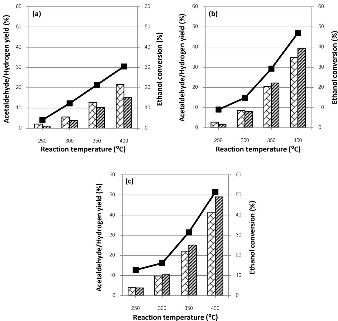
**Figure 4.9** Ethanol conversion, acetaldehyde and hydrogen yield as a function of reaction temperature for ethanol dehydrogenation reaction over 2.5 wt.% Cu-Ag/SiO<sub>2</sub> (a), 5 wt.% Cu-Ag/SiO<sub>2</sub> (b) and 10 wt.% Cu-Ag/SiO<sub>2</sub> (c) catalyst prepared by typical impregnation technique (■ ethanol conversion, □ acetaldehyde yield and ▨ hydrogen yield)
