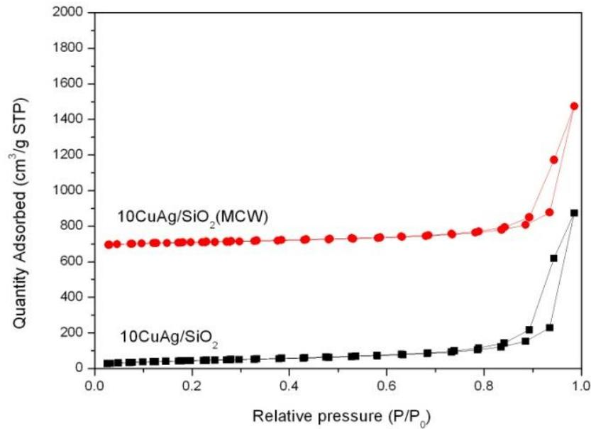
**Figure B.10** Adsorption and desorption isotherms of 10 wt.% copper and silver doped on silica support: (■) typical impregnation technique and (●) microwave-assisted technique.
