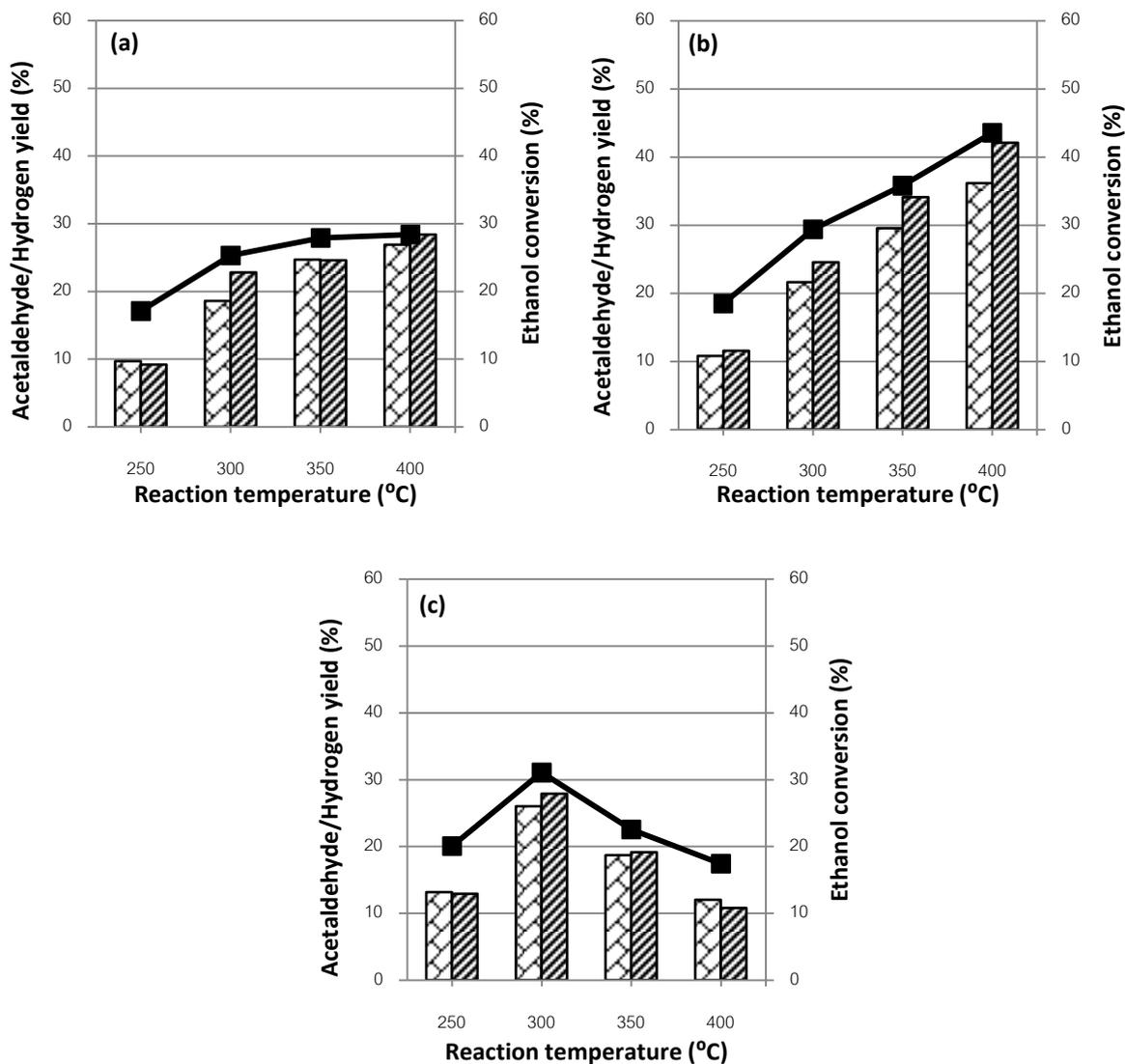
**Figure 4.10** Ethanol conversion, acetaldehyde and hydrogen yield as a function of reaction temperature for ethanol dehydrogenation reaction over 2.5 wt.% Cu/SiO<sub>2</sub> (a), 5 wt.% Cu/SiO<sub>2</sub> (b) and 10 wt.% Cu/SiO<sub>2</sub> (c) catalyst prepared by microwave-assisted technique (■ ethanol conversion, ▨ acetaldehyde yield and ▩ hydrogen yield).
