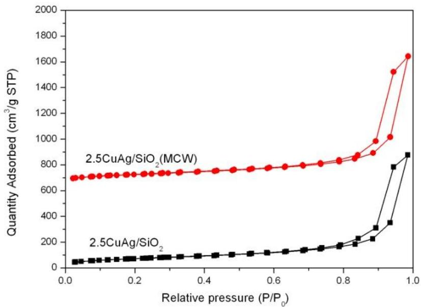
**Figure B.4** Adsorption and desorption isotherms of 2.5 wt.% copper and silver doped on silica support: (■) typical impregnation technique and (●) microwave-assisted technique.
