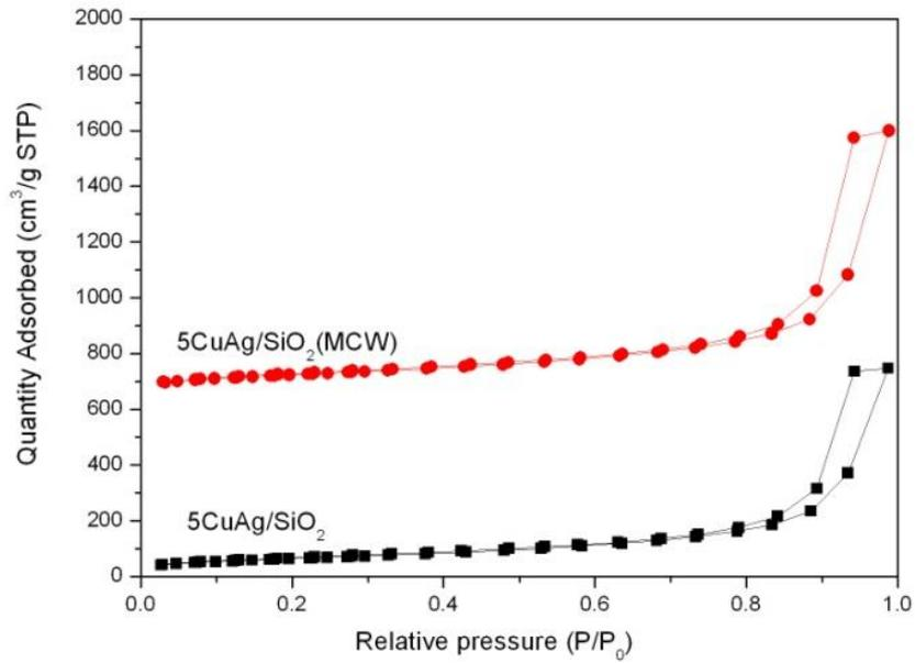
**Figure B.7** Adsorption and desorption isotherms of 5 wt.% copper and silver doped on silica support: (■) typical impregnation technique and (●) microwave-assisted technique.
