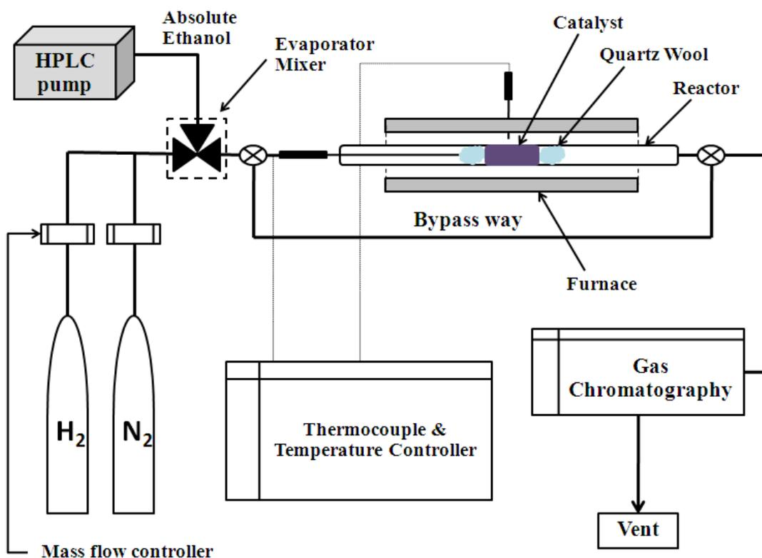
**Figure 3.3** Schematic diagram of catalytic dehydrogenation of ethanol system.
