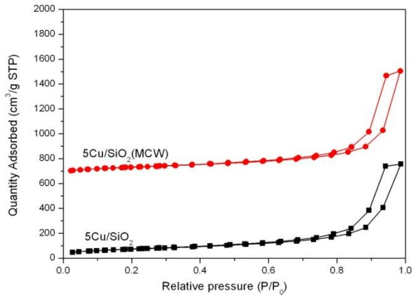
**Figure B.5** Adsorption and desorption isotherms of 5 wt.% copper doped on silica support: (■) typical impregnation technique and (●) microwave-assisted technique.
