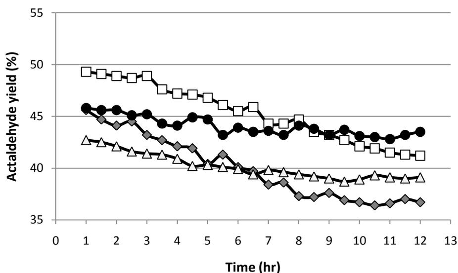
**Figure 4.13** Acetaldehyde yield as a function of time over synthesized catalyst for dehydrogenation of ethanol operated at 400°C (◆ 10 wt.% Ag/SiO<sub>2</sub>, ▲ 10 wt.% Cu-Ag/SiO<sub>2</sub> prepared by typical impregnation technique, and ■ 10 wt.% Ag/SiO<sub>2</sub>, ● 10 wt.% Cu-Ag/SiO<sub>2</sub> prepared by microwave-assisted technique).
