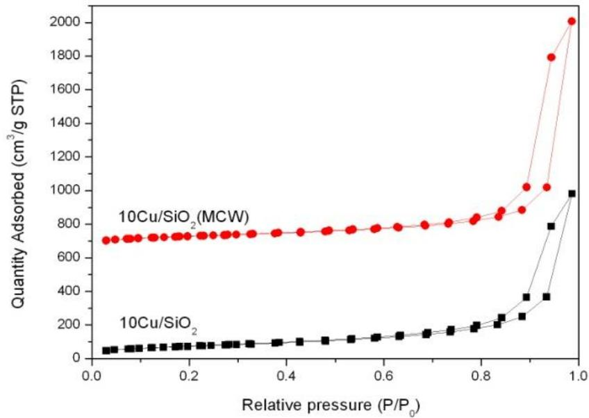
**Figure B.8** Adsorption and desorption isotherms of 10 wt.% copper doped on silica support: (■) typical impregnation technique and (●) microwave-assisted technique.
