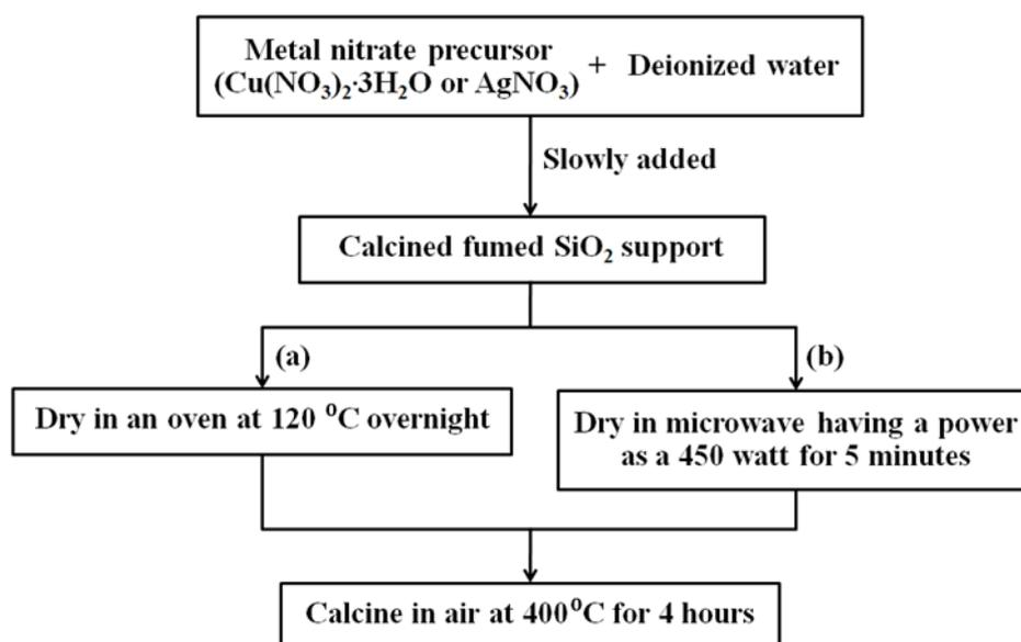
**Figure 3.2** Schematic diagram of catalyst preparation by (a) impregnation technique and (b) microwave-assisted technique.
