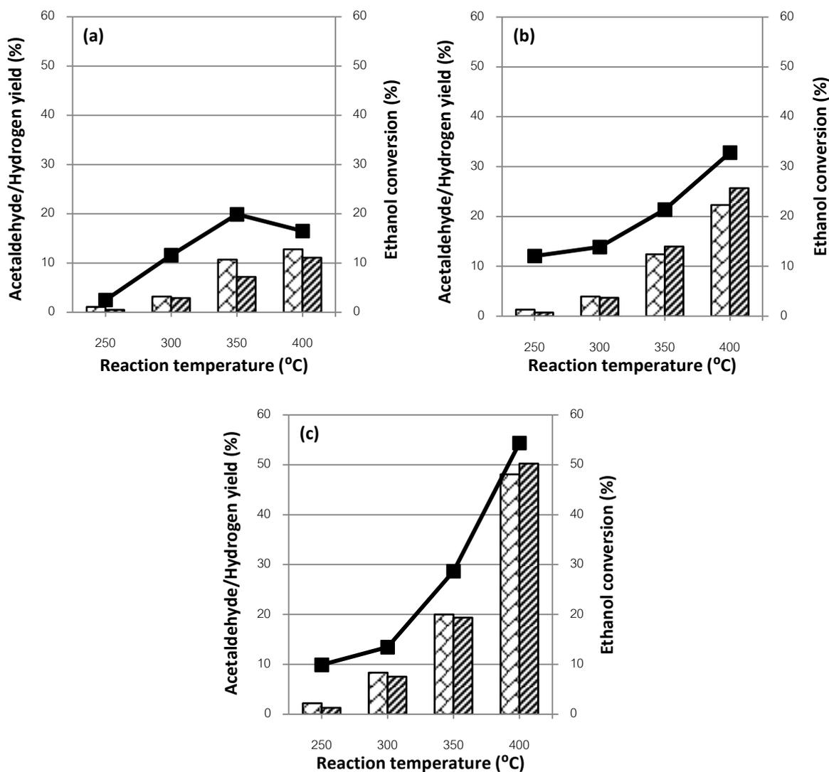
**Figure 4.11** Ethanol conversion, acetaldehyde and hydrogen yield as a function of reaction temperature for ethanol dehydrogenation reaction over 2.5 wt.% Ag/SiO<sub>2</sub> (a), 5 wt.% Ag/SiO<sub>2</sub> (b) and 10 wt.% Ag/SiO<sub>2</sub> (c) catalyst prepared by microwave-assisted technique (■ ethanol conversion, □ acetaldehyde yield and ▨ hydrogen yield).
