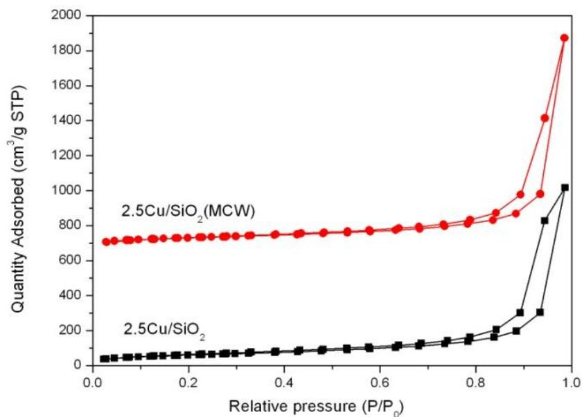
**Figure B.2** Adsorption and desorption isotherms of 2.5 wt.% copper doped on silica support: (■) typical impregnation technique and (●) microwave-assisted technique.
