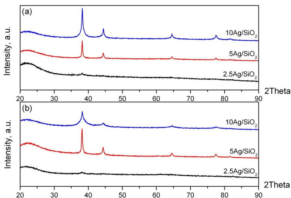
**Figure 4.2** XRD patterns of silver doped on silica support catalyst after reduced in 10% v/v H<sub>2</sub> in N<sub>2</sub> at 300°C for 3 hours at different silver loadings: (a) typical impregnation technique and (b) microwave-assisted technique.
