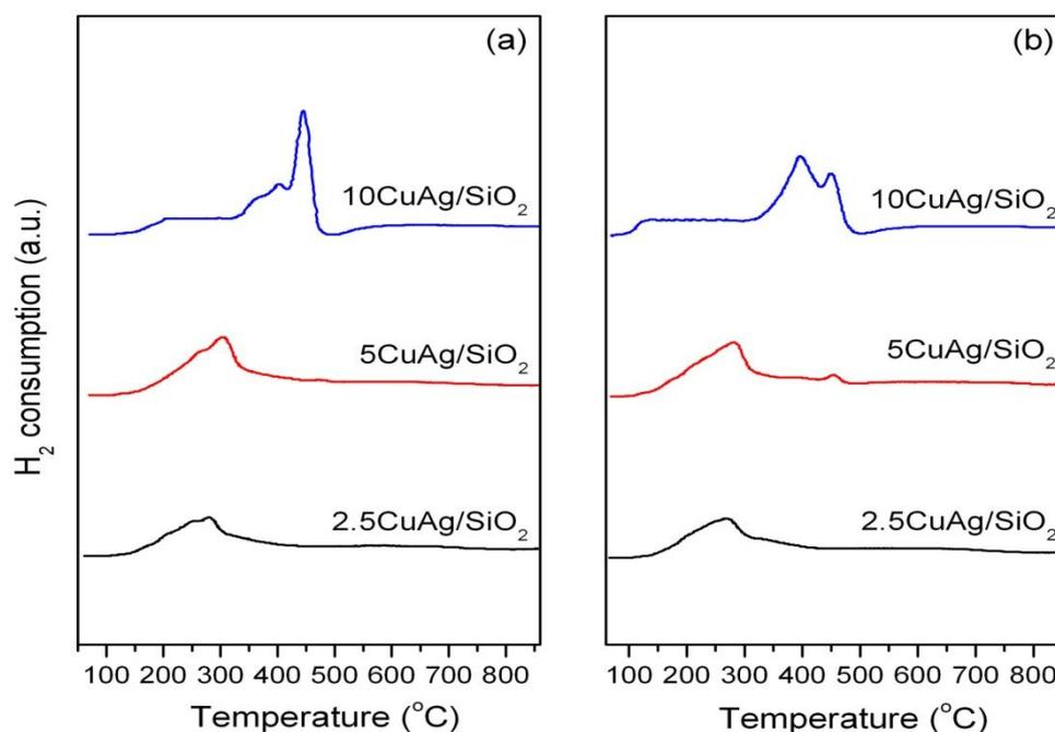
**Figure 4.6** TPR profiles of bimetallic copper and silver doped on silica support catalyst at different total metal loadings: (a) typical impregnation technique and (b) microwave-assisted technique.
