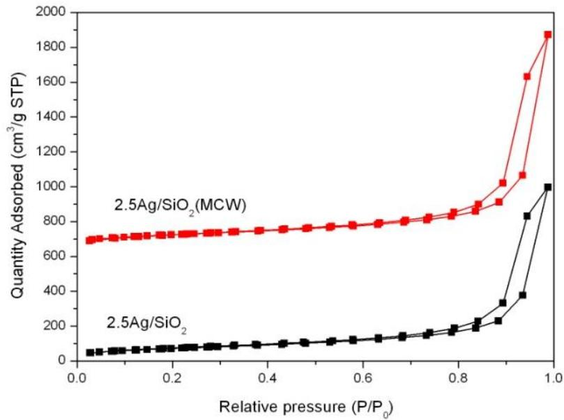
**Figure B.3** Adsorption and desorption isotherms of 2.5 wt.% silver doped on silica support: (■) typical impregnation technique and (●) microwave-assisted technique.
