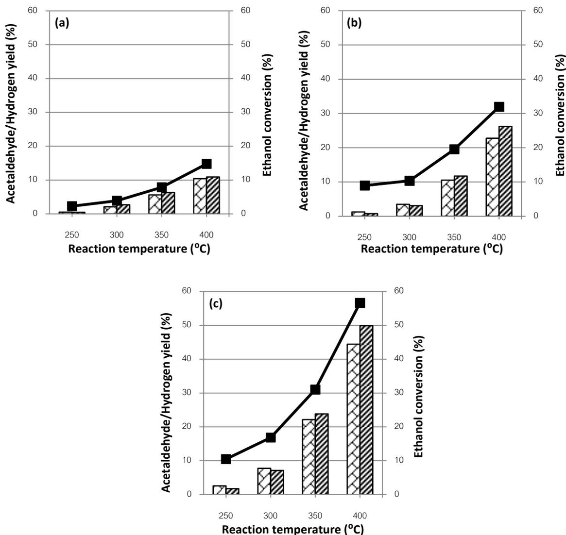
**Figure 4.8** Ethanol conversion, acetaldehyde and hydrogen yield as a function of reaction temperature for ethanol dehydrogenation reaction over 2.5 wt.% Ag/SiO<sub>2</sub> (a), 5 wt.% Ag/SiO<sub>2</sub> (b) and 10 wt.% Ag/SiO<sub>2</sub> (c) catalyst prepared by typical impregnation technique (■ ethanol conversion, □ acetaldehyde yield and ▨ hydrogen yield).
