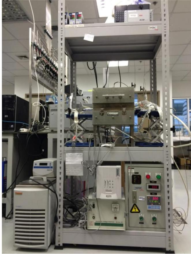
**Figure 3.4** Catalytic dehydrogenation of ethanol system.
