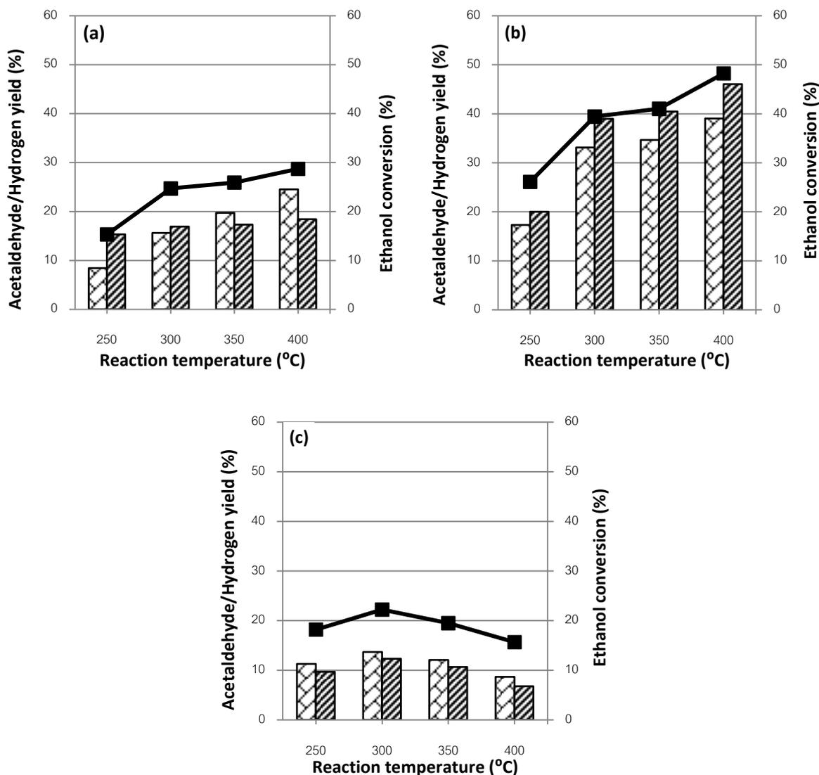
**Figure 4.7** Ethanol conversion, acetaldehyde and hydrogen yield as a function of reaction temperature for ethanol dehydrogenation reaction over 2.5 wt.% Cu/SiO<sub>2</sub> (a), 5 wt.% Cu/SiO<sub>2</sub> (b) and 10 wt.% Cu/SiO<sub>2</sub> (c) catalyst prepared by typical impregnation technique (■ ethanol conversion, □ acetaldehyde yield and ▨ hydrogen yield).
