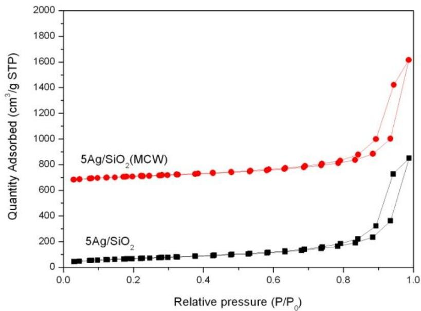
**Figure B.6** Adsorption and desorption isotherms of 5 wt.% silver doped on silica support: (■) typical impregnation technique and (●) microwave-assisted technique.
