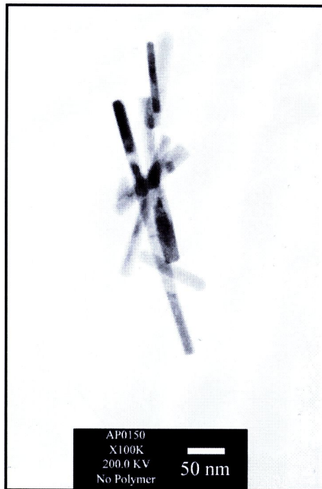
Figure 3.67 TEM image of \text{Bi}_2\text{S}_3 hydrothermally produced in polymer-free solution at 200 °C, 20 h
