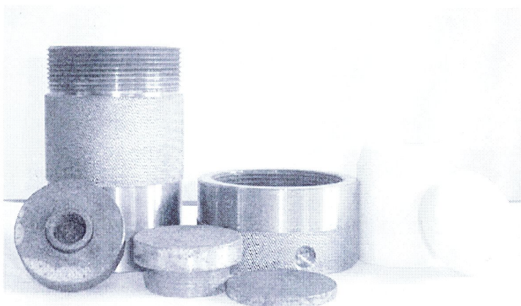
Figure 1.11 General purpose autoclave popularly used for hydrothermal synthesis
