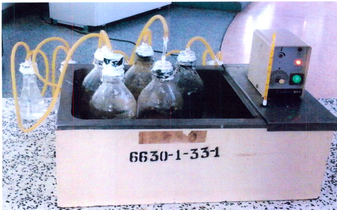
Figure 6 Experiment on the influence of particle size on biogas production set up
