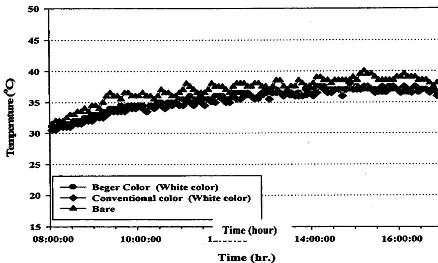
**Figure 37 (d) Comparing envelop at the inside eastern wall surface show room temperature of small building coated with high solar reflective paint, conventional color and uncoated**
