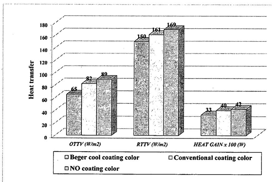
**Figure 46 Representations a comparison between overall heat transfers in to the building painted with Beger Cool, conventional paint, and no coating**
