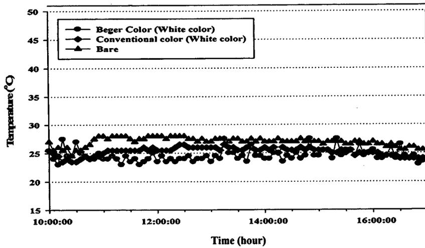
**Figure 38 (e) Comparing envelop at the center of room show room temperature of small building coated with high solar reflective paint, conventional color and uncoated**
