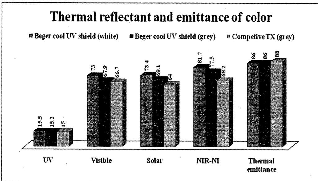
**Figure 44 The percentile of thermal reflectance and emittance of different type of paint**
