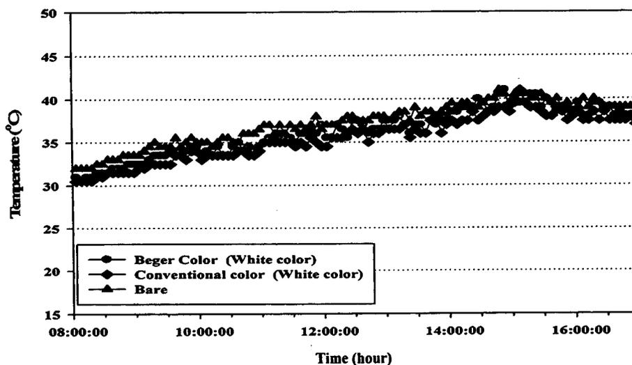
**Figure 36 (c) Comparing envelop at the outside eastern wall surface show room temperature of small building coated with high solar reflective paint, conventional color and uncoated**
