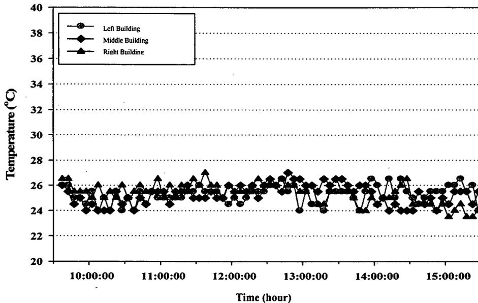
**Figure 33 (d) The effect of building location on envelop surface and of room temperature (Based case) at the center of room**
