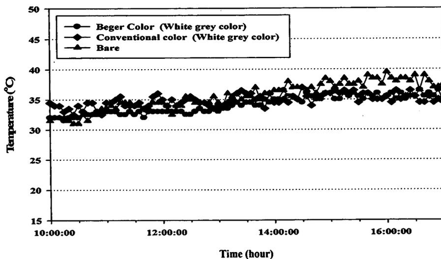
**Figure 42 (i) Comparing envelop at the inside eastern wall surface show room temperature of small building coated with high solar reflective paint, conventional color and uncoated**
