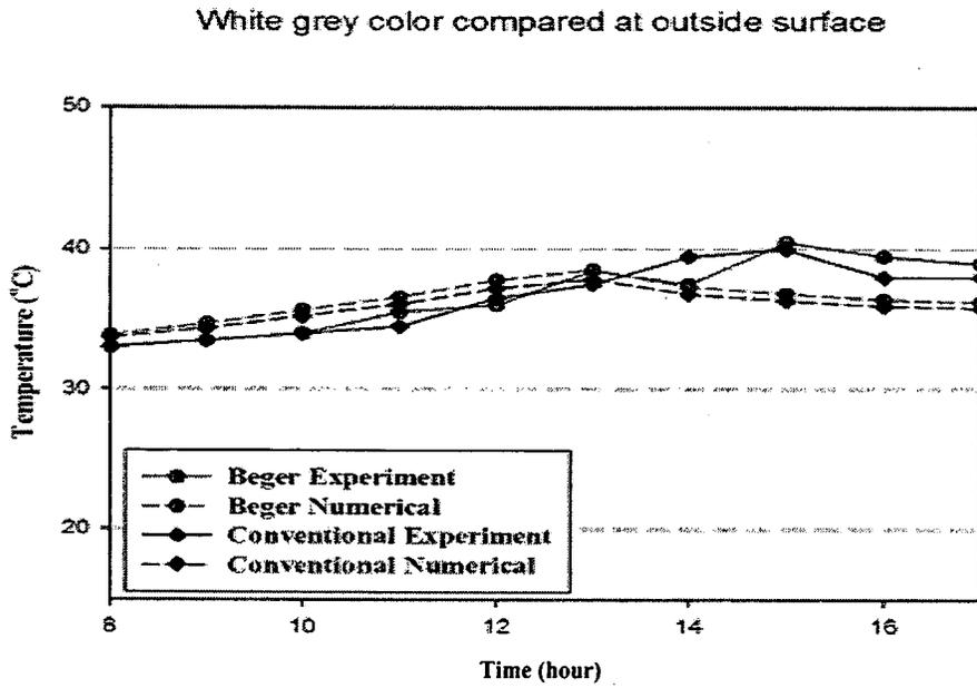
**Figure 49 (c) Comparing outside wall temperature surface of numerical and experimental result**
