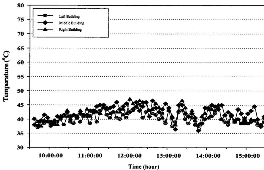
**Figure 32 (c) The effect of building location on envelop surface and of room temperature (Based case) at the outside roof surface on the first day**
