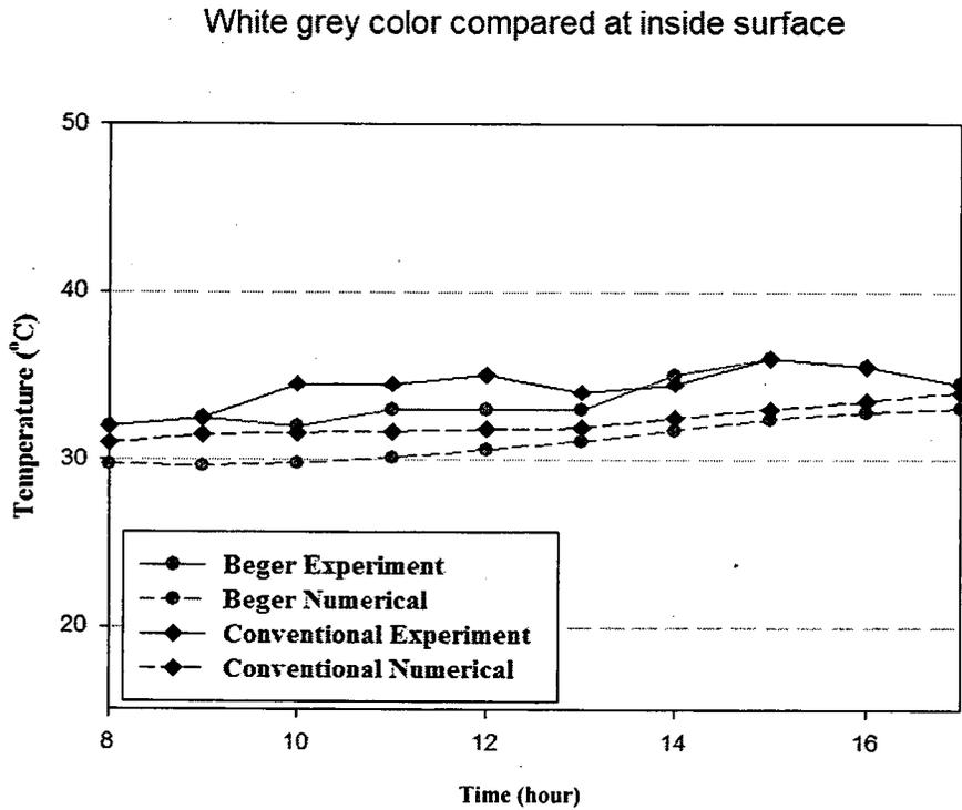
**Figure 50 (d) Comparing inside wall temperature surface of numerical and experimental result**
