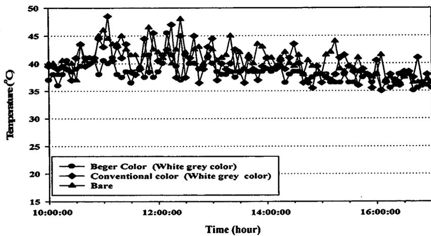
**Figure 39 (f) Comparing envelop at the outside roof surface show room temperature of small building coated with high solar reflective paint, conventional color and uncoated**
