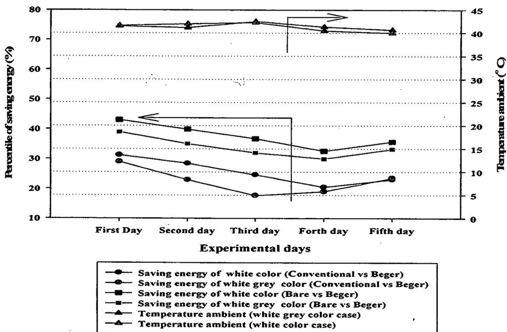
Figure 45 The comparing percentile of saving energy of small building coated with white and white grey color
