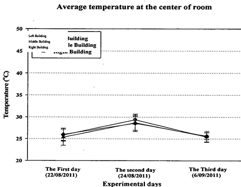
**Figure 30 (a) The effect of building location on envelop surface and of room temperature (Based case) at center of the room**
