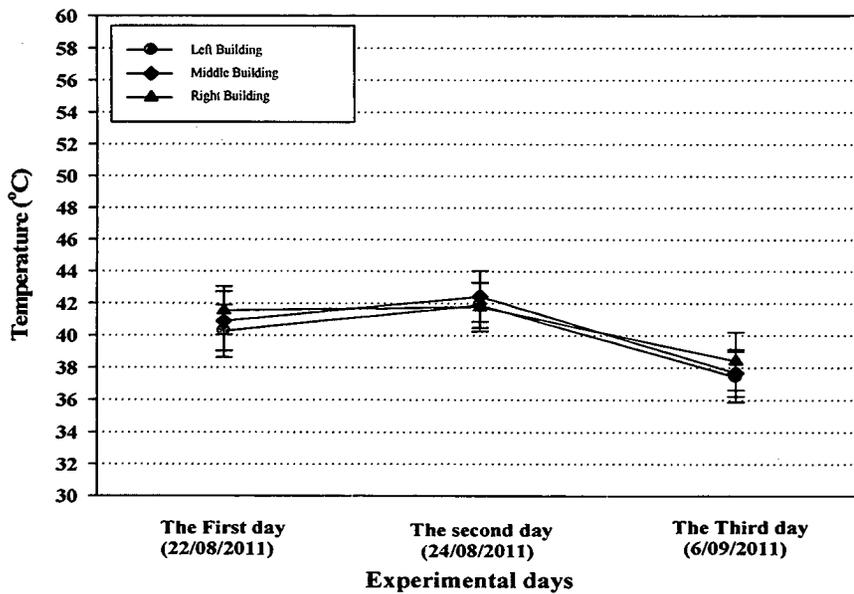
**Figure 31 (b) The effect of building location on envelop surface and of room temperature (Based case) at the outside roof surface of room**
