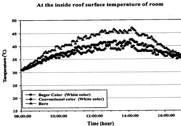
**Figure 35 (b) Comparing envelop at the inside roof show surface room temperature of small building coated with high solar reflective paint, conventional color and uncoated**
