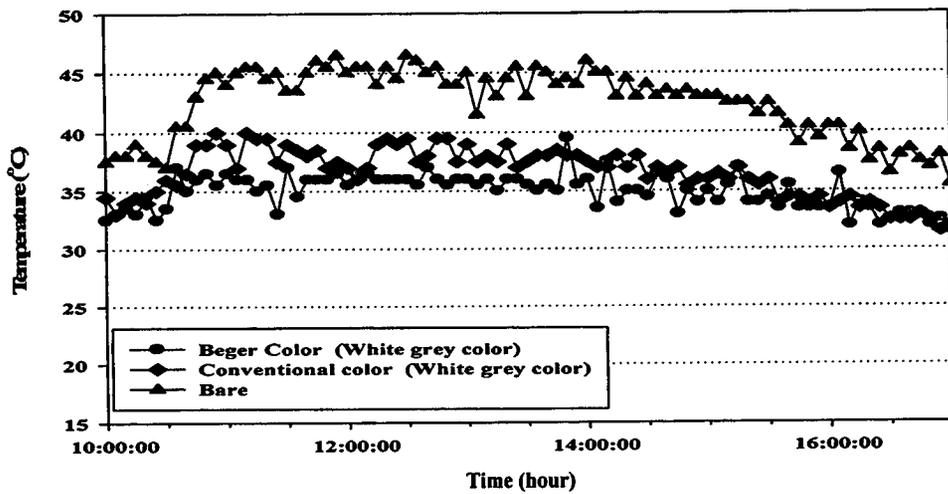
**Figure 40 (g) Comparing envelop at the inside roof surface show room temperature of small building coated with high solar reflective paint, conventional color and uncoated**
