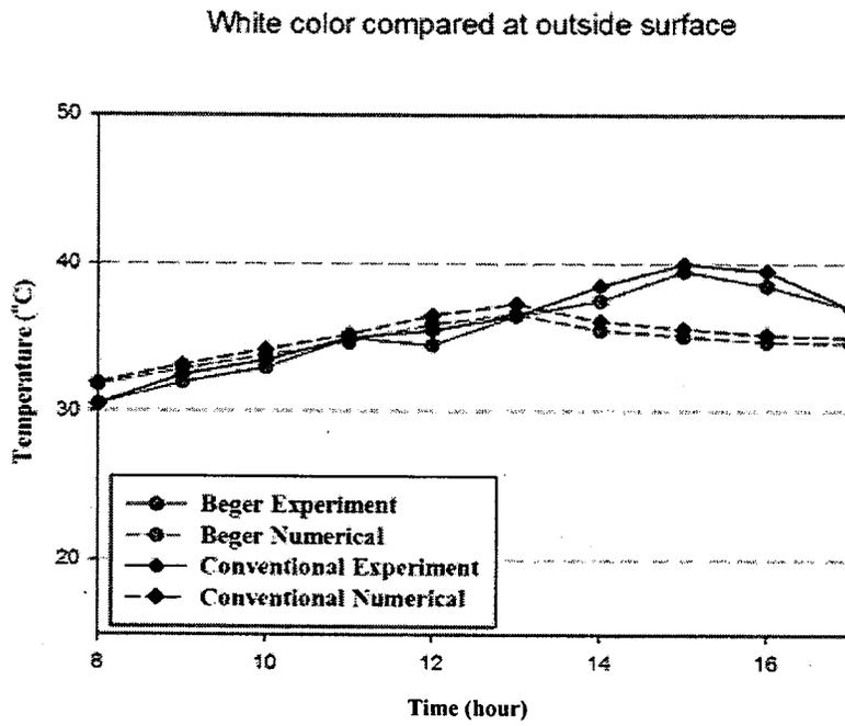
**Figure 47 (a) Comparing outside wall temperature surface of numerical and experimental result**
