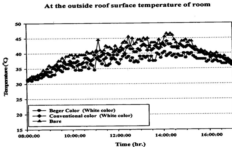
**Figure 34 (a) Comparing envelop at the outside roof surface show room temperature of small building coated with high solar reflective paint, conventional color and uncoated**
