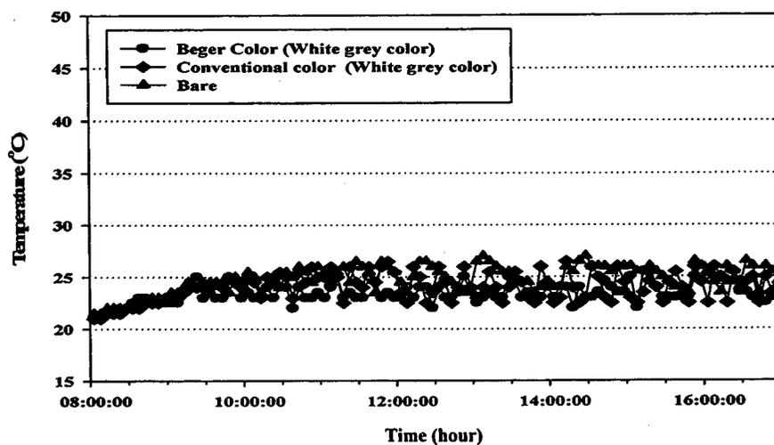
**Figure 43 (j) Comparing envelop at the of the room show room temperature of small building coated with high solar reflective paint, conventional color and uncoated**
