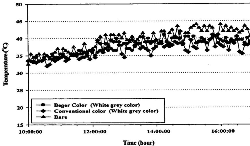
**Figure 41 (h) Comparing envelop at the outside eastern wall surface show room temperature of small building coated with high solar reflective paint, conventional color and uncoated**
