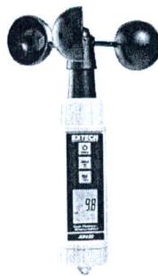
**Figure 24 Cup anemometer**
