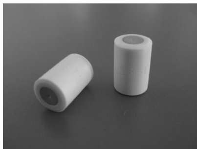
Figure B2 Guard column Zorbax SB-C18, 1.25 cm length, 4.6 mm i.d. and 5 \mu\text{m} (Agilent Technologies, USA)
