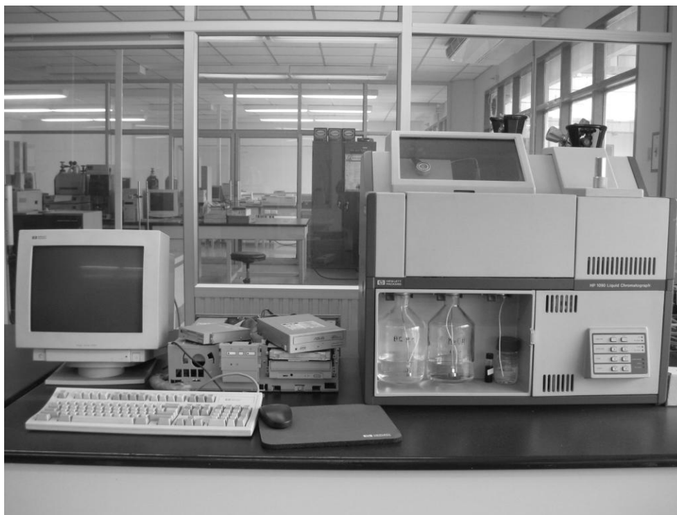
Figure B1 High performance liquid chromatograph (HP 1090A, Agilent Technologies, USA)
