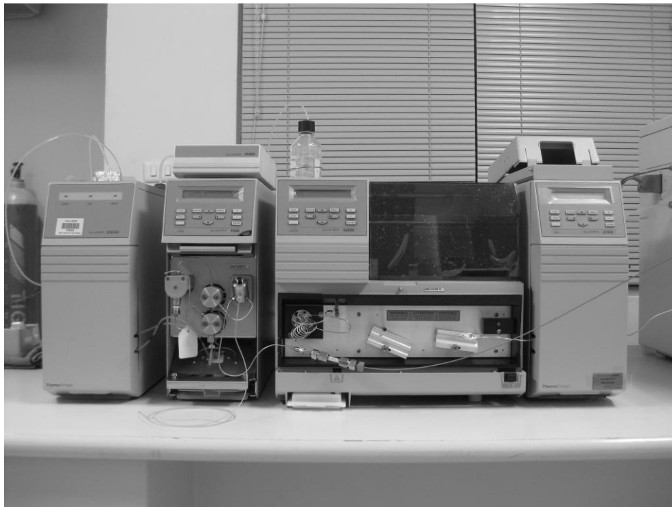
Figure B3 High performance liquid chromatograph (SpectraSYSTEM, Thermo Finnigan, USA)
