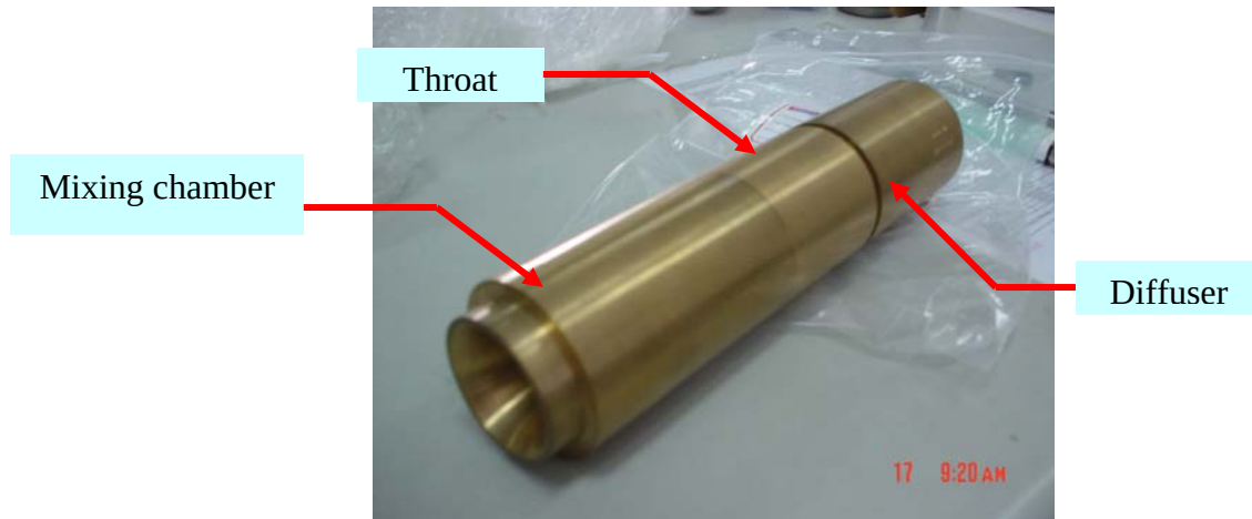
Figure 3.6 Photograph of an ejector used in the experiment.
