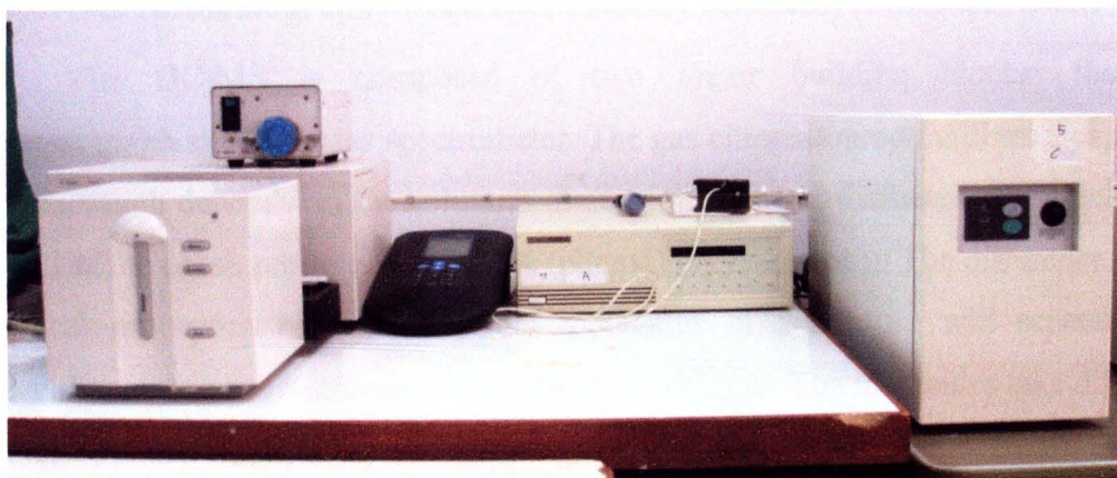
Figure A1 Agilent Model 8453 spectrophotometer; an UV-visible spectrophotometer
