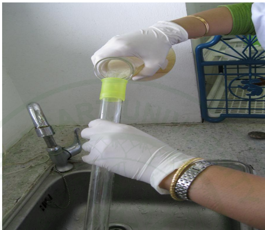
Figure 7 Collection of the Amberlite XAD-16 bounded with CFNS in the column.
