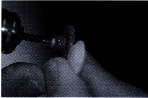
Figure 18 The core-veneer specimen was ground using a green stone bur
