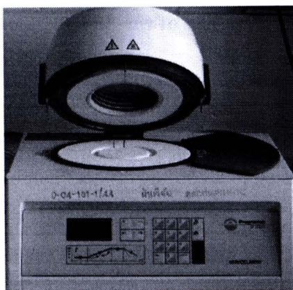
Figure 6 The Programmat P100 furnace (Ivoclar-Vivadent, Schaan, Liechtenstien) that was used for porcelain firing
