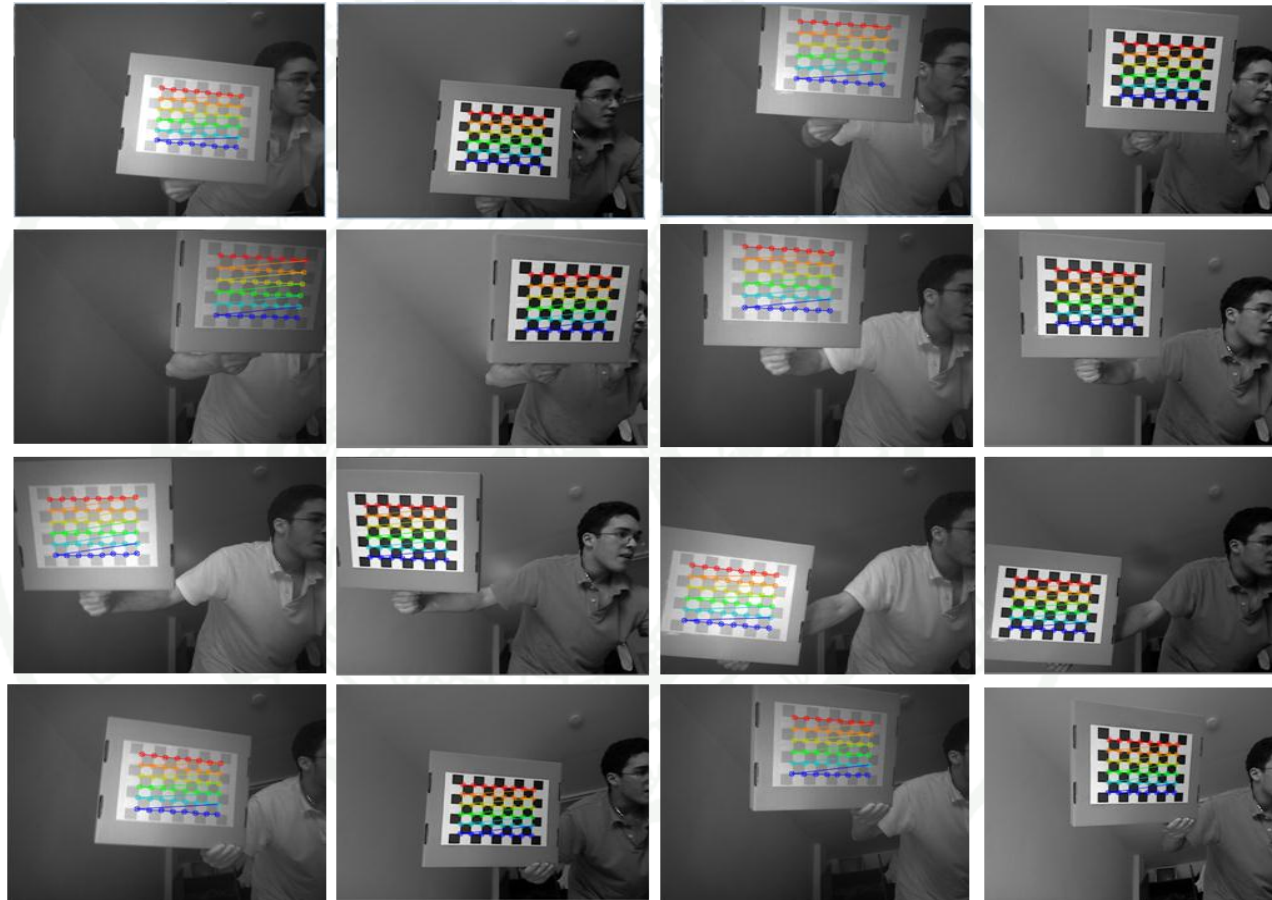
Figure 52 Extract black-white-black-white features 48 points on chessboard that upper images are captured from the depth camera and lower images are captured from the color camera (There are 16 images: 8 depth images and 8 color images).
