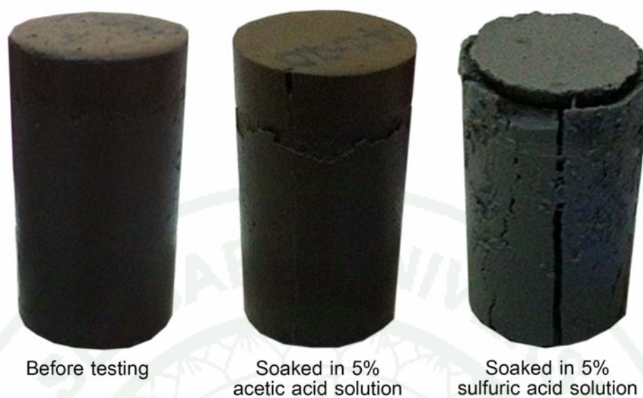
Appendix Figure B1 Visual appearance of 10C-70 geopolymer paste for class C fly ash before and after exposure to 5% solutions of acetic and sulfuric acids after 18 weeks
