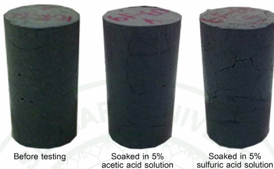
Appendix Figure B3 Visual appearance of 10F-60 geopolymer paste for class F fly ash before and after exposure to 5% solutions of acetic and sulfuric acids after 18 weeks.
