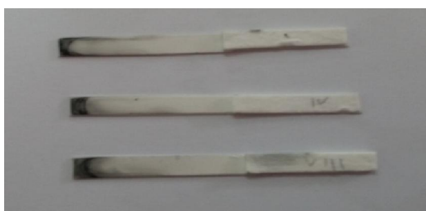
Figure 4.5 Flow of 0.2% (w/v) antibody-carbon nanoparticle conjugate on the membrane where various concentrations of NGAL protein were spotted at 1 \mu\text{L}/\text{spot} .
