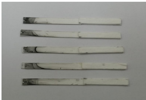
Figure 4.4 Flow of 0.2% (w/v) antibody-carbon nanoparticle conjugate with a concentration on the membrane previously spotted with various concentrations of NGAL protein at 2 \mu\text{L}/\text{spot} .
