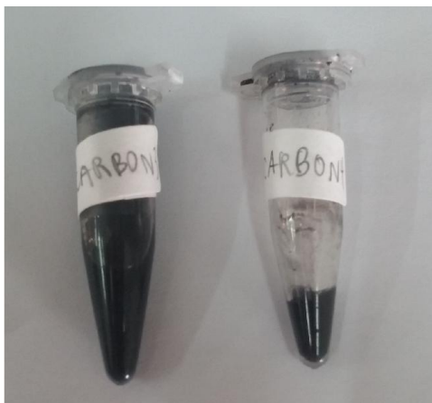
Figure 4.15 Varying the ratio of carbon suspension and antibody at 2000:1 (left) and 667: 1 (right).
