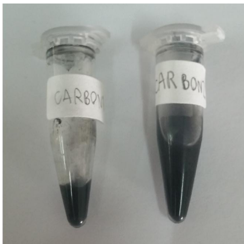
Figure 4.11 Varying the ratio of carbon suspension and antibody at 5000:1 in using different stirring speeds: 150 rpm (left) and 200 rpm (right).
