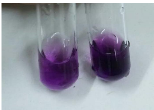
Figure 4.7 The color intensity of the highest concentration of BSA standard curve (40 µg/ml) and sample.
