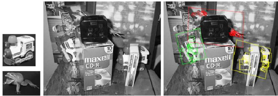
Figure 2.11 Example of SURF The training images for two objects are shown on the left. These can be recognized in a cluttered image with extensive occlusion, shown in the middle. The results of recognition are shown on the right[27].
