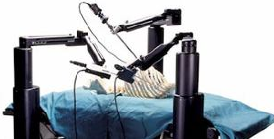
Figure 2.1 Three robotic arms of the Zeus surgical system [15]
