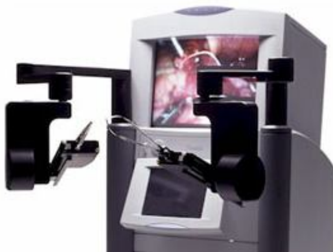
Figure 2.2 Surgeon Console of the Zeus surgical system [15]
