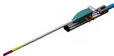
Figure 6. Bending laparoscope External Manipulator Part
