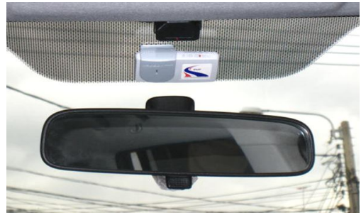
Figure 2.14 EASY PASS Card install at windshield Source: Expressway Authority of Thailand (2010)
