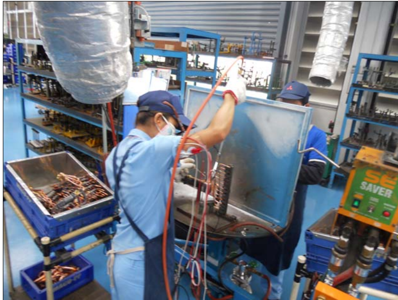
Figure 2.16 Copper capillary tube welding posture
