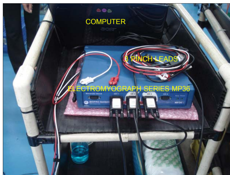
Figure C-2 Show Computer, Electromyograph series MP36 acquisition unit and 3 Pinch leads
