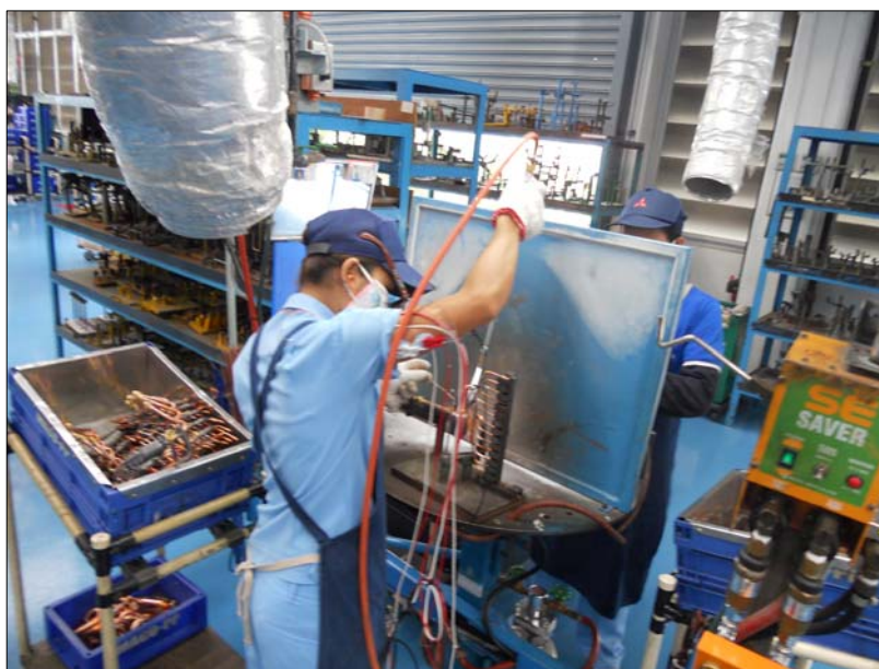
Figure C-6 Show posture by usage of existing torch to weld
