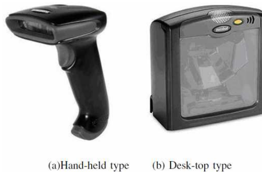
Figure 2.7 Two types of common laser bar-code readers
