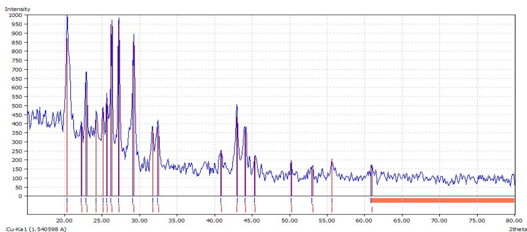
Figure 5-31: Permanent Yellow paint diffractogram matched to reference in the model database
