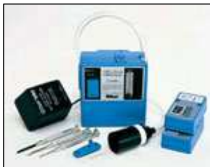
Figure 3-9 Apparatus for collection of dust samples
