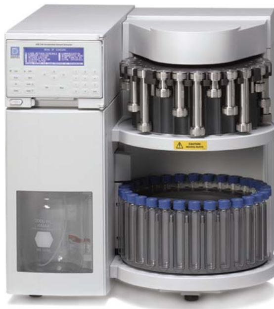
Figure 2.4: Accelerated Solvent Extraction, DIONEX ASE200 model
