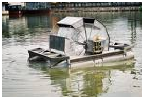
Chai Pattana Aerator
