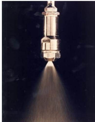
**Figure 2.8** Atomizer in operation (Nozzle atomizer)
