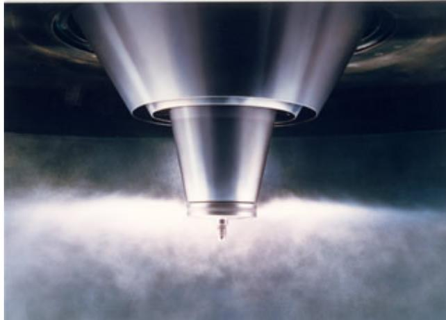
**Figure 2.7** Atomizer in operation (Rotary atomizer)
