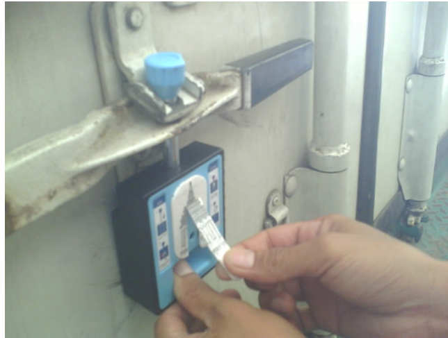
Figure 4.6 E-seal unlock for opening goods container door
