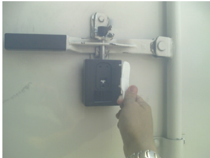
Figure 4.4 Process of locking e-seal at container truck
