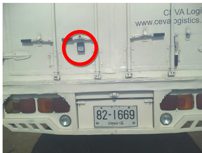
Figure 4.5 Container truck has been already locked by e-seal
