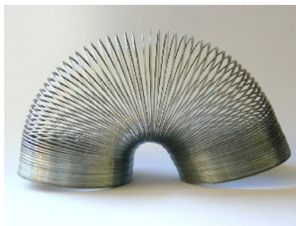
Slinky for the longitudinal wave demonstration
